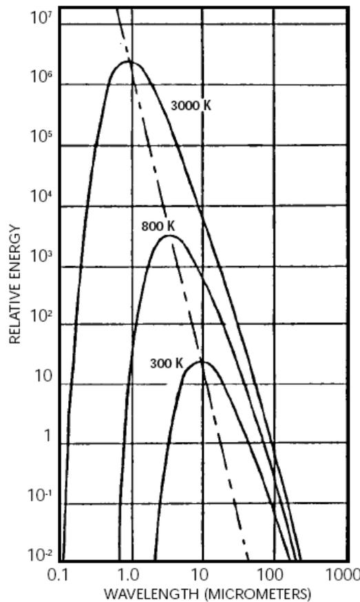
Fig.1: Radiation intensity as a function of wavelength and temperature (Planck's Law)
