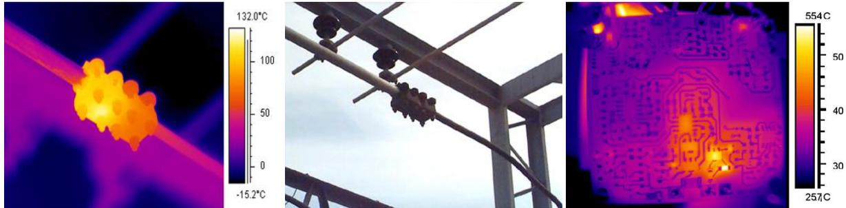
Picture 1: a) Bolted connection problem b) PC board with overheating component.
