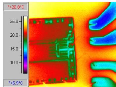
Picture 2: Thermal image of a microcircuit showing 7 micron leads.
