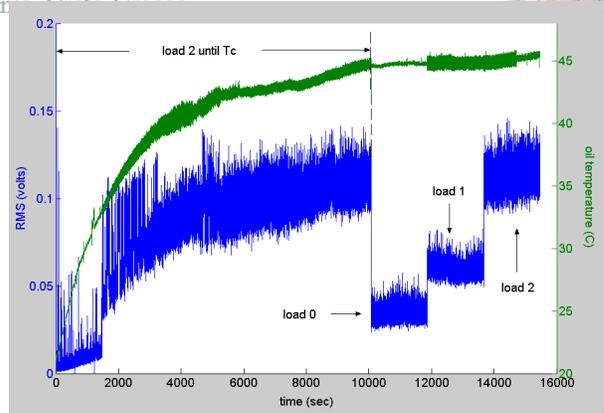
Figure 6: RMS level for defect [C] - all loads
