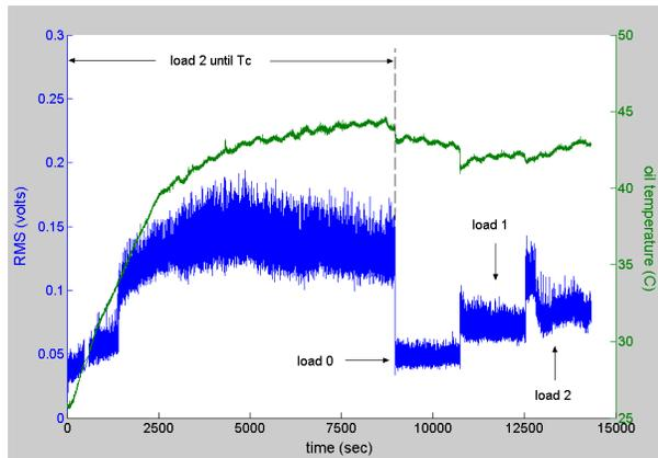
Figure 4: RMS level for defect [A] - all loads
