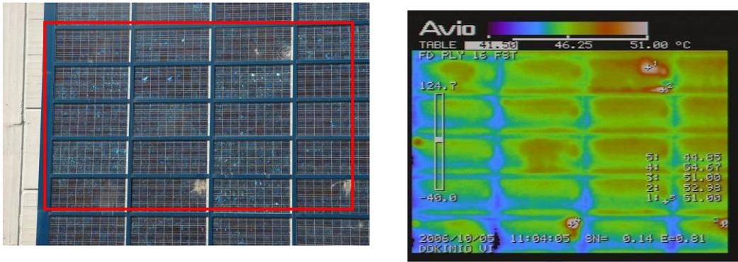
Figure 3 : Hot spot detection. The particular spots are the result of vandalism
