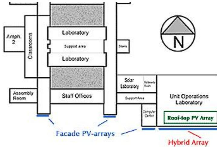
Figure 1 : Ground plan of Chemical Engineering Building where PV arrays are placed
