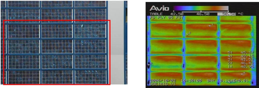
Figure 6 : Horizontal temperature gradients in the modules
