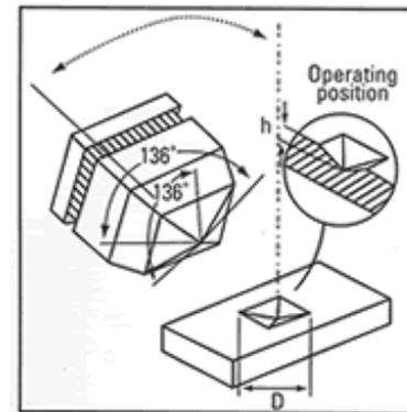
Figure 2: Schematic presentation of Vickers probe and its indentation
