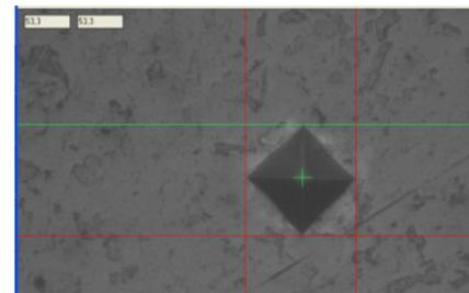
Fig.11. The 21<sup>st</sup> Indentation up to the core (40x).
