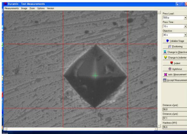
Fig. 6 The reference block test indentation [18]
