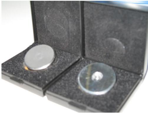
Fig. 5 Micro Vickers Reference Hardness Blocks
