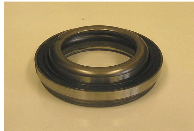
Figure 5 Tested axial bearing (external diameter 60mm, internal 35mm, 15 rolling elements - balls)
