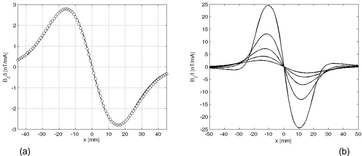
Fig.3 Coil in air. (a) Variation of  $B_z$  as a function of distance  $x$  across the excitation coil at a vertical distance of 28.9mm. Circles are measurements and straight lines represent theoretical calculations. (b) The same variation for five different distances from the coil ranging from  $z=10$ mm to 30mm in steps of 5mm.
