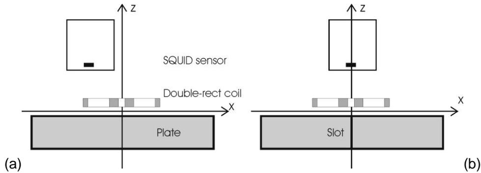
Fig.2 Magnetic field measurement using a SQUID sensor (a) Excitation coil in air or above plate without defect, only the SQUID sensor is moved (b) Coil above plate with defect, SQUID sensor and excitation coil are moved together.
