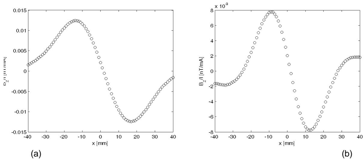
Fig.6 Coil and sensor above long subsurface slot in a plate conductor, variation of  $B_z$  as a function of  $x$ . (a) Real and (b) Imaginary part of experimental results.
