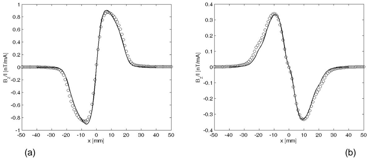
Fig.5 Coil and sensor above long through thickness slot in a plate conductor, variation of  $B_z$  as a function of  $x$ . (a) Real and (b) Imaginary part. Circles are measurements and straight lines represent theoretical calculations.
