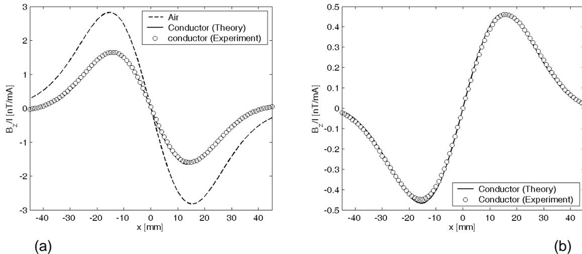
Fig.4 Coil in air and above conductive plate. Variation of  $B_z$  as a function of distance  $x$  across the excitation coil at a vertical distance of 28.9mm (a) Real part and (b) Imaginary part of total magnetic field. Circles are measurements and straight lines represent theoretical calculations. Note the decrease in the total magnetic field due to the conductive plate.
