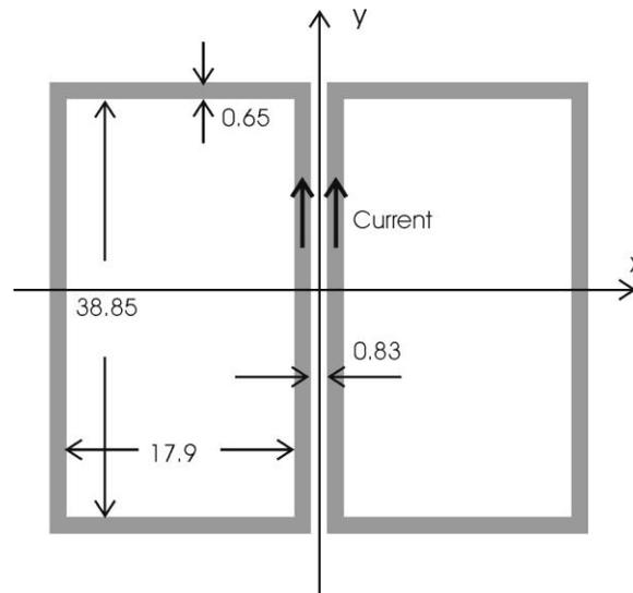
Fig.1 Top view of the double-rectangle PCB coil that was used as excitation. The copper layer thickness is  $30\mu\text{m}$ .
