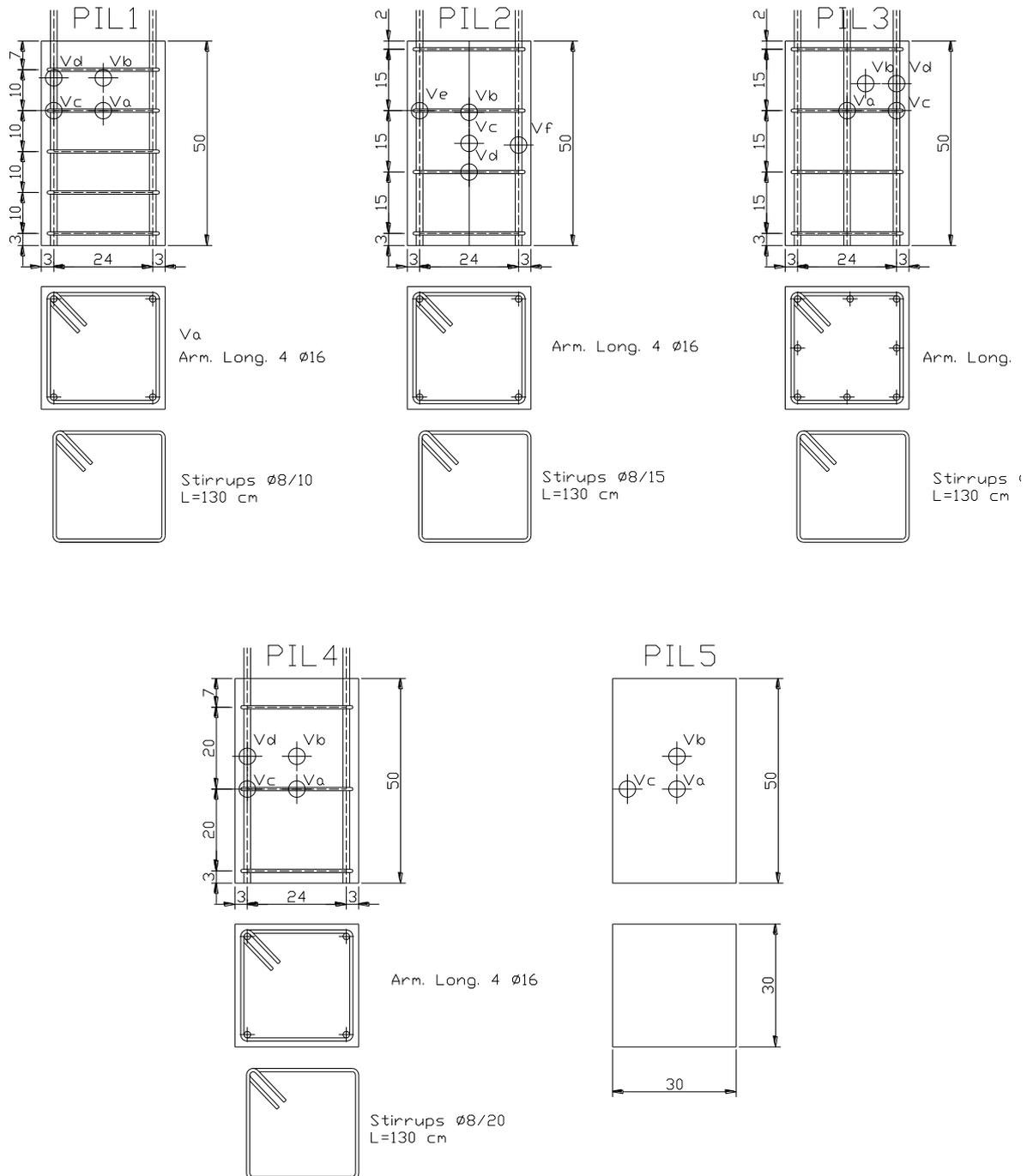
Figure 3: Points of Ultrasonic Pulse Velocity measurement
