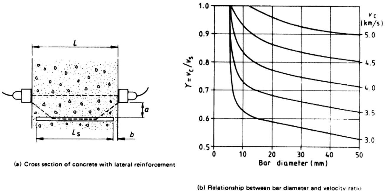
Figure 1: BS 1881-203-1986 - Influence of steel reinforcement on pulse velocity (bar parallel to pulse path) [2]
