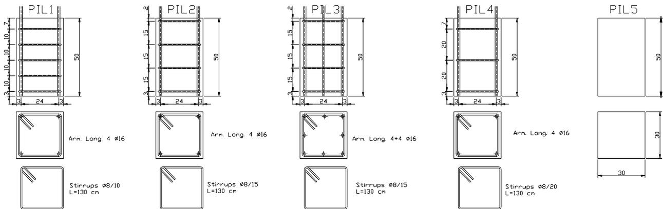
Figure 2: Reinforced concrete and concrete Specimens
