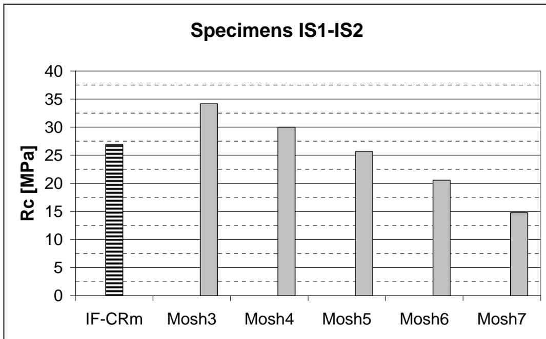
Figure 5. Specimens IS – Correlation between “Windsor Strength and core strength
