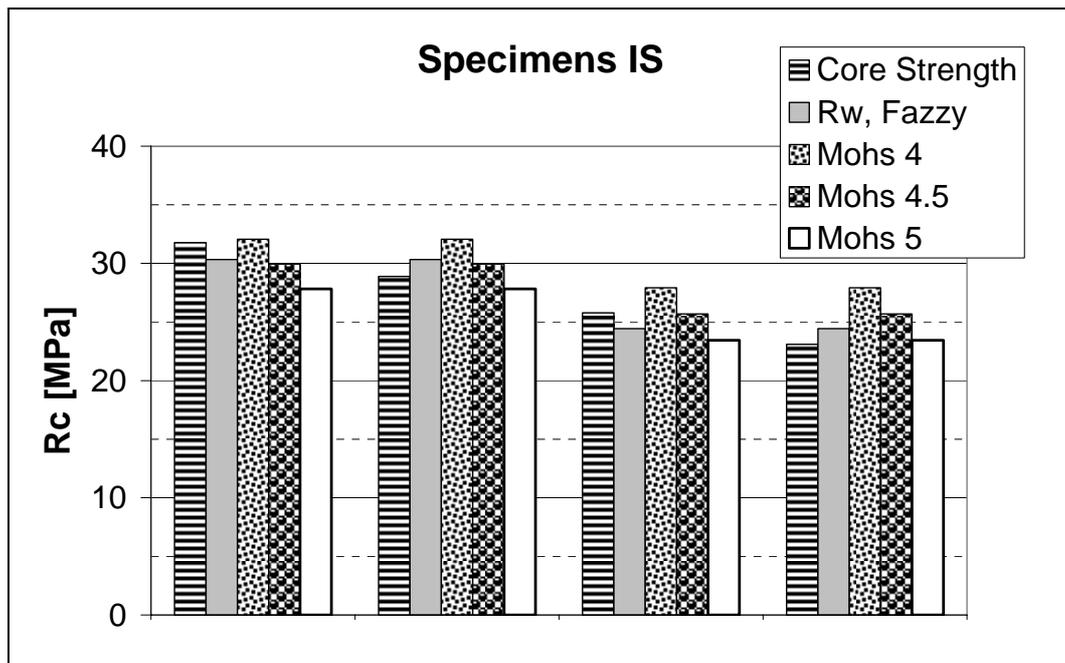
Figure 7. Specimens IS – Correlation among “Windsor Strength”, “Fuzzy Strength” and Core Strength
