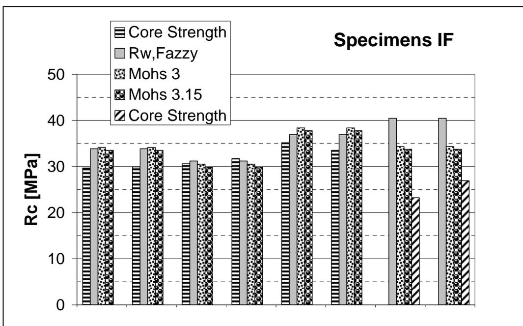
Figure 6. Specimens IF – Correlation among “Windsor Strength”, “Fuzzy Strength and Core Strength
