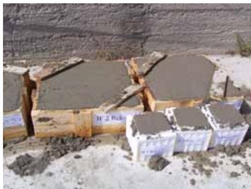
Figure 2. Specimens IF - Mohs'hardness variable from 3 to 7
