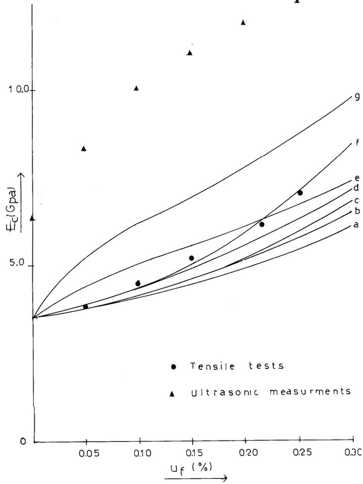
**Fig. 3.** The elastic modulus  $E_c$  versus filler volume fraction in epoxy/iron particulate composites
