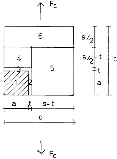
**Fig. 1.** A Schematic representation of the square-into-square model taking into account the interface. Model 1.
