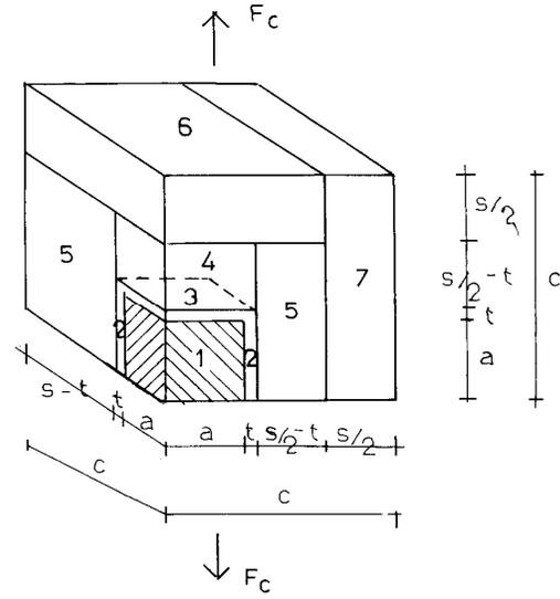
**Fig. 2.** A Schematic representation of the cube-within-cube model taking into account the interface. Model 2.
