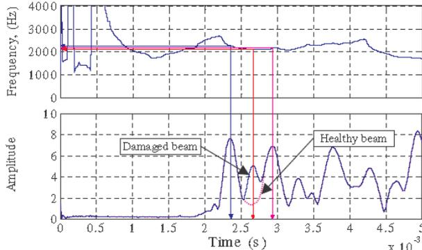
Figure 2- Amplitude-time plot of the sensor response [3]
