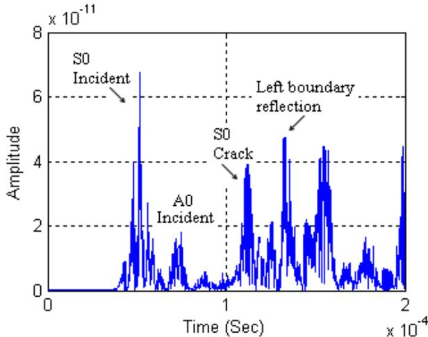
Figure 12-Energy density level versus time plot of sensor response obtained from HHT analysis
