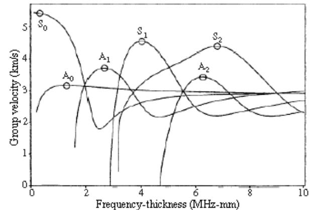
Figure 4- The group dispersion curve for aluminum plate
