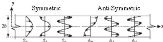
Figure 3-The first few fundamental lamb wave modes for propagation within a plate of thickness 2b [4],[7]
