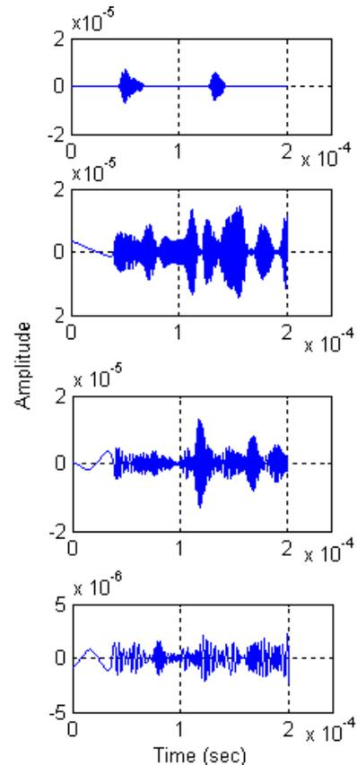
Figure 11- First four IMFs for response signal of horizontal actuation force.
