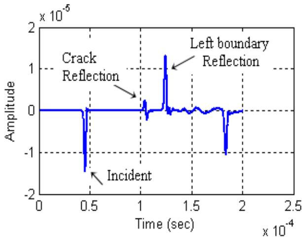
Figure 9- Sensor response caused by horizontal impact actuation
