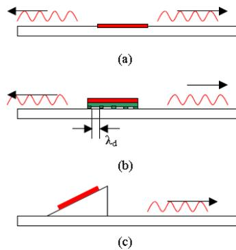
Figure 6- Methods for lamb wave generation. a) using Y-cut piezoelements.b) using X-cut piezoelements with predefined spacing c) using inclined piezoelectric probe.[8]
