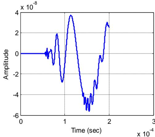
Figure 8- sensor response caused by vertical impact actuation
