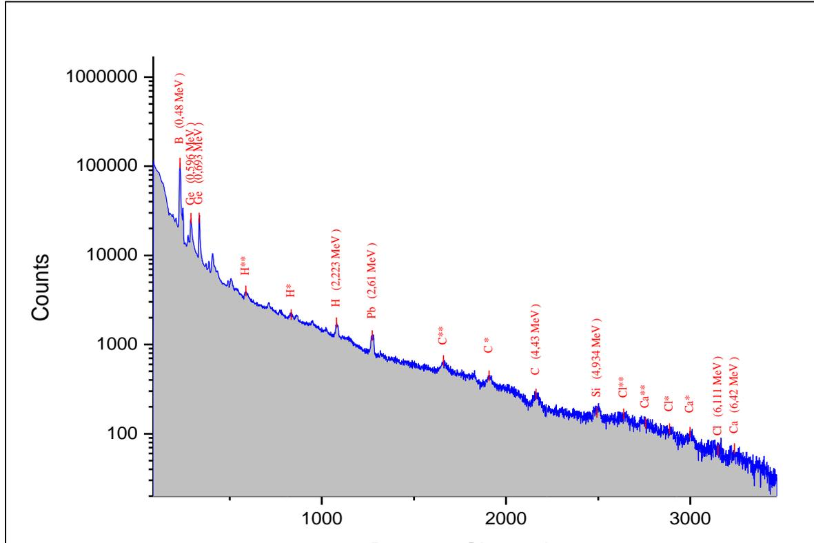
Figure 2 : PGNAA spectrum of concret, in the photon energy range 0 – 7 MeV
