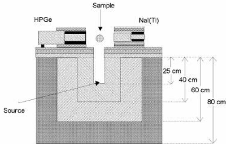
Figure 1 : PGNAA schematic diagram
