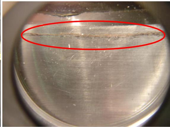
Corrosion with depth of 0.2 mm (2)
