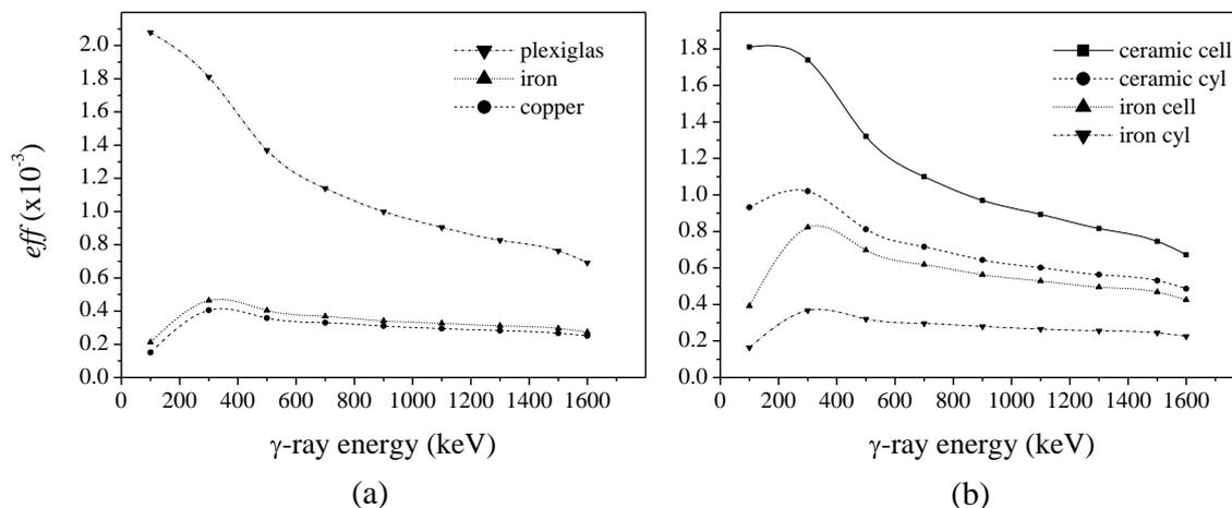
Figure 6 : Predicted detector efficiency as a function of gamma ray energy for (a) slab samples composed of Plexiglas, iron and copper and (b) cylindrical cell and cylindrical samples composed of ceramic and iron
