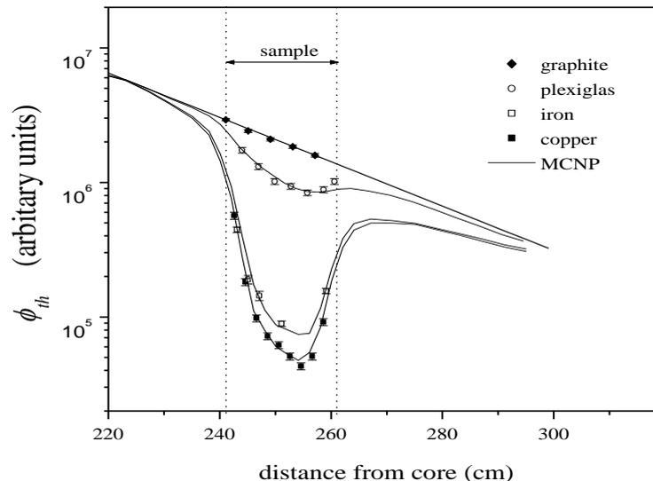
Figure 4 : Thermal neutron flux distribution in slab samples composed of Plexiglas, iron and copper, as a function of distance from the reactor core
