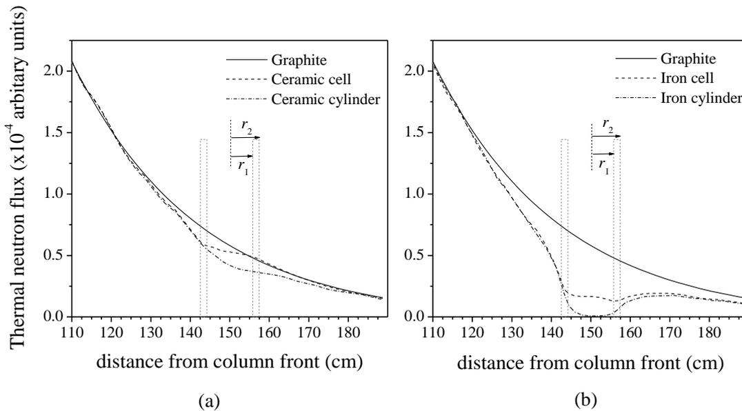
Figure 5 : Predicted thermal neutron flux distribution as a function of distance in the presence of cylindrical cell and cylindrical samples composed of (a) ceramic and (b) iron
