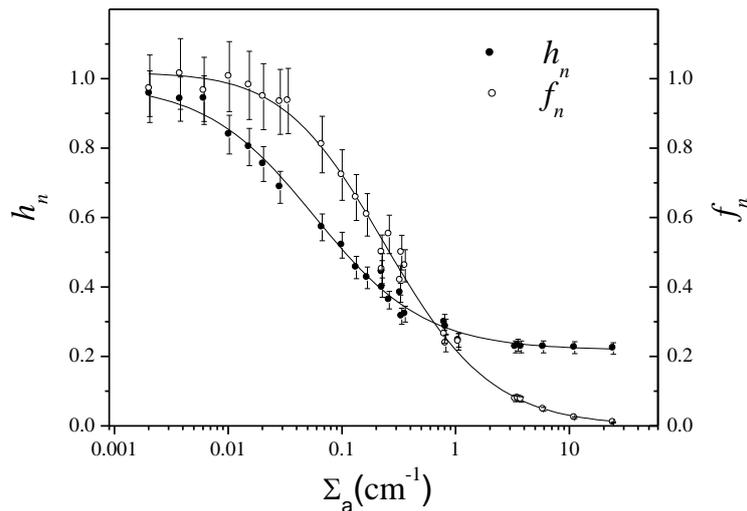
Figure 2 : Thermal neutron flux depression factor ( $h_n$ ) and self-shielding factor ( $f_n$ ) as a function of the macroscopic thermal neutron absorption cross-section ( $\Sigma_a$ ) of cylindrical samples 5 cm in radius and 20 cm in height
