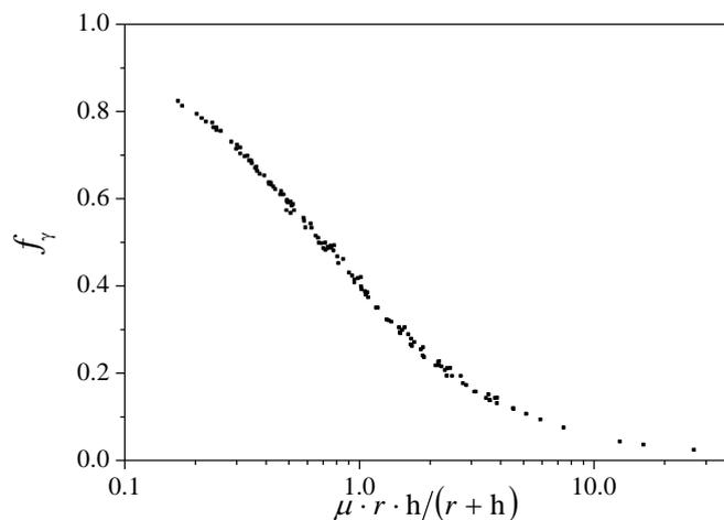
Figure 3 : Predicted volume source efficiency correction factor,  $f_\gamma$ , as a function of the dimensionless variable  $\mu \cdot r \cdot h / (r + h)$
