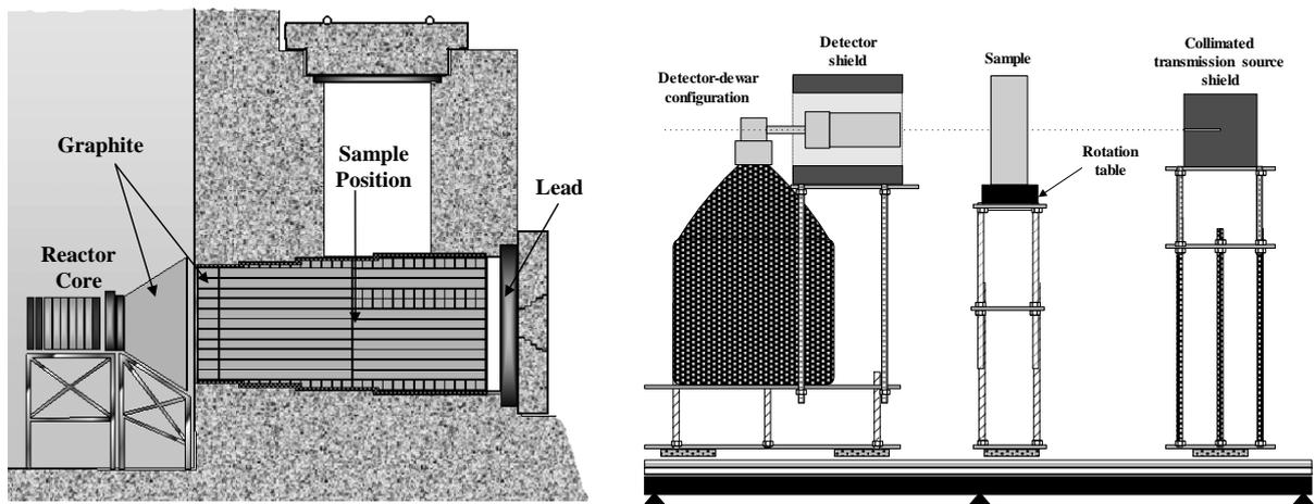
Figure 1 : Schematic representation of (a) the GRR-1 core and graphite column irradiation facility and (b) spectroscopy and transmission measuring facility (vertical cross-sections)
