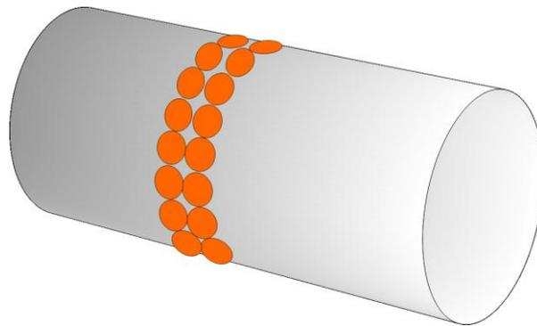
Fig 2 A typical eddy current probe array around a tube.
