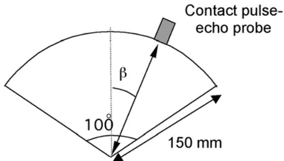
Figure 4. Experimental set-up for measuring wedge diffraction coefficients.  $\beta$  is the angle to the wedge bisector and is the angle plotted on the horizontal axes of Figures 5 and 6 below
