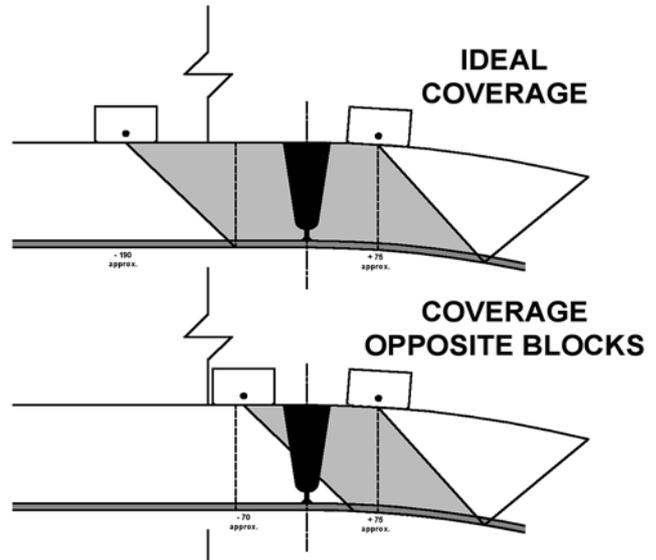
Figure 9. Example of scan restriction due to support lugs: 45° probe up scan to half skip
