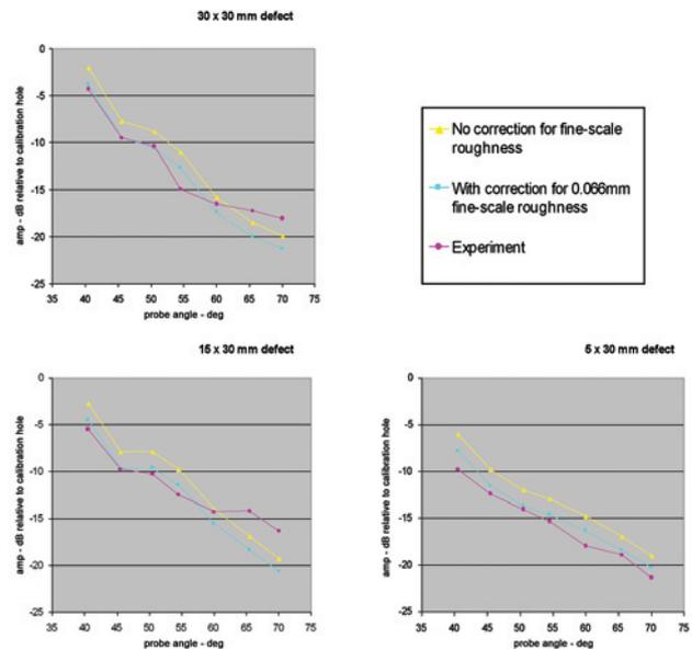
Figure 2. Pulse-echo responses from three different rough defects with 7 different probe beam angles: comparison between experiment and globally corrected TRANGLE code predictions. All three defects are tilted by 50°, so the 40° probe gives normal incidence on the defects
