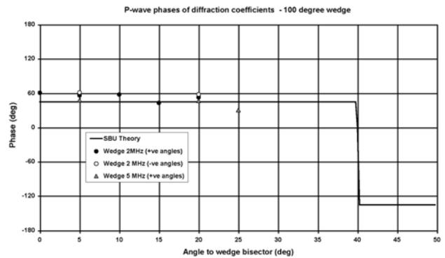
Figure 6. Phases of back-scattered wedge diffraction coefficients for compression waves in a 100° vertex: comparison between experiment (plotted points) and LSBU theory (solid curve)
