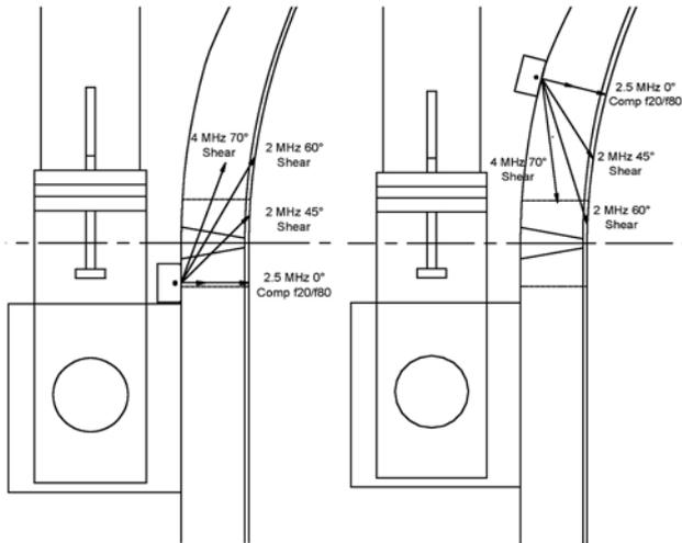
Figure 7. Scan design for Sizewell B pressuriser weld inspection: half-skip up scans (left) and half-skip down scans (right)
