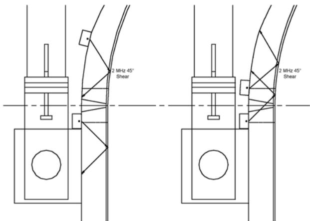
Figure 8. Scan design for Sizewell B pressuriser weld inspection: full-skip down scans (left) and full-skip up scans (right)
