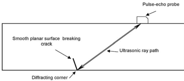
Figure 3. Diffraction from a corner for surface-breaking cracks
