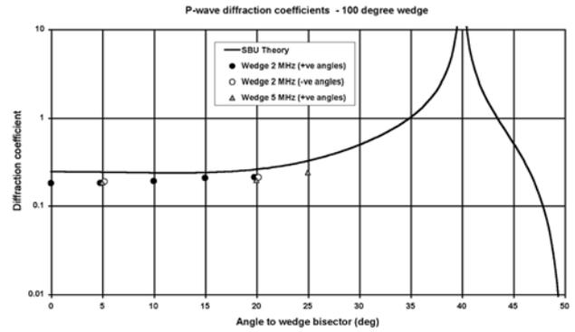
Figure 5. Amplitudes of back-scattered wedge diffraction coefficients for compression waves in a 100° vertex: comparison between experiment (plotted points) and LSBU theory (solid curve)
