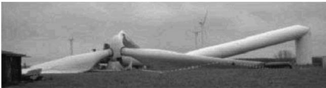
Figure 4. Collapsed wind turbine tower due to fatigue cracks and wind loading combination
