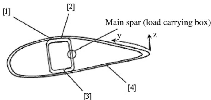
Figure 2. Sketch of section of blade (local coordinates) Risø
