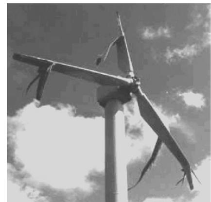
Figure 3. Delamination of the blades
