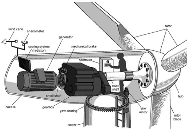
Figure 1. Wind turbine open nacelle (from Danish Wind Industry Association)
