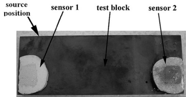
**Figure 5. Sensor and source positions for source location measurement**
