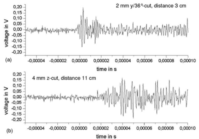
**Figure 6. Acoustic emission signals in time domain detected by (a) sensor 1 (2 mm  $y/36^\circ$ -cut piezocomposite) 3 cm from source; (b) sensor 2 (4 mm z-cut) 11 cm from source**
