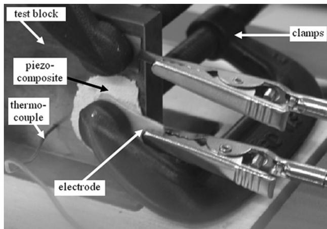
Figure 2. Lithium niobate piezocomposite mounted onto the test object (metal block standing vertically on hotplate)
