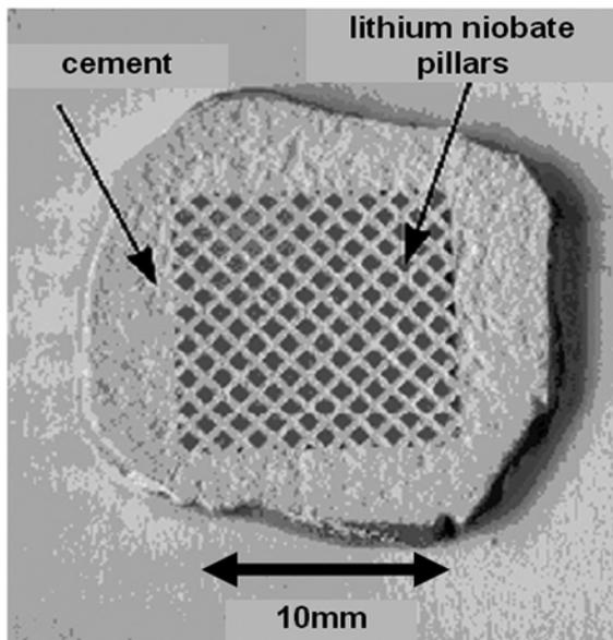
Figure 1. Lithium niobate cement piezocomposite with pillar width 0.8 mm and volume fraction of lithium niobate 45%
