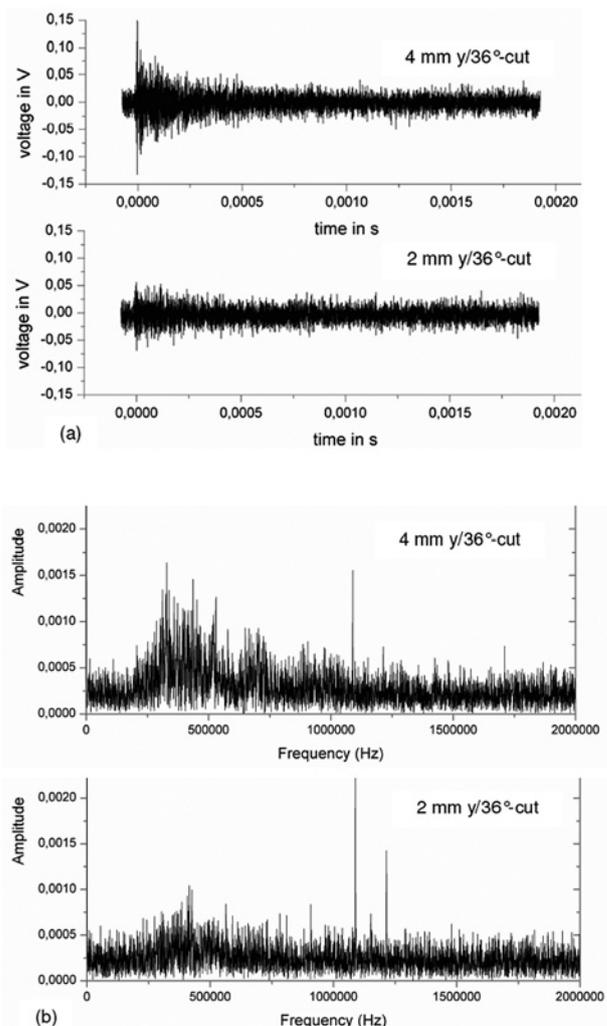
Figure 3. Comparison between 4 mm and 2 mm-thick y/36°-cut piezocomposites: (a) acoustic emission signal in time domain; (b) frequency spectrum. The 4 mm-thick transducer is more sensitive at low frequencies, due to its lower resonant frequency
