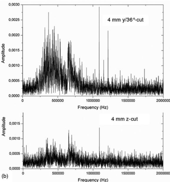
**Figure 4. Comparison between 4 mm-thick  $y/36^\circ$ -cut and z-cut piezocomposites: (a) acoustic emission signal in time domain; (b) frequency spectrum. The  $y/36^\circ$ -cut transducer has greater sensitivity due to a larger  $k_t$ .**
