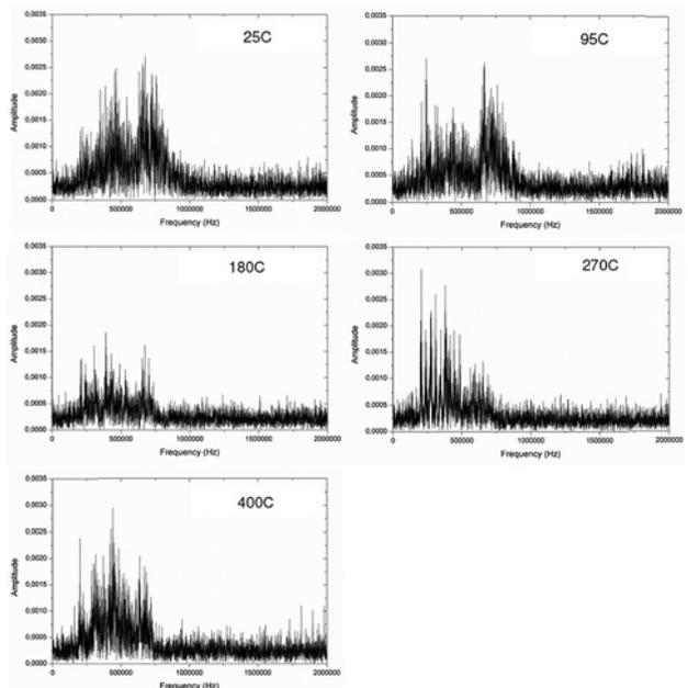
**Figure 7. 4 mm-thick  $y/36^\circ$ -cut piezocomposite, frequency spectrum measured at temperatures up to 400°C with 3 cm between sensor and source**
