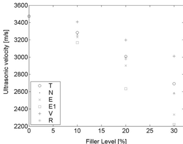
Figure 9. Ultrasonic velocity versus filler level
