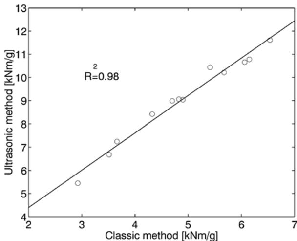
Figure 12. Stiffness obtained with classic and ultrasonic methods
