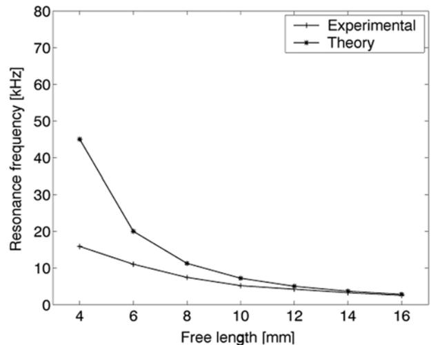
Figure 6. Resonance frequency versus free length
