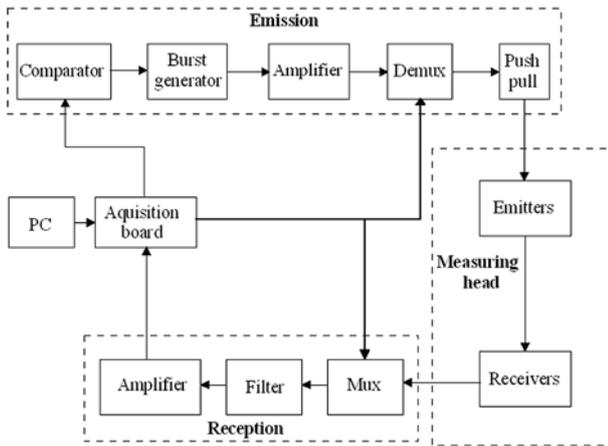
Figure 8. Schematic diagram of the system
