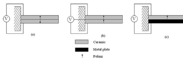
Figure 3. Schematic configuration of bimorphs and unimorphs
