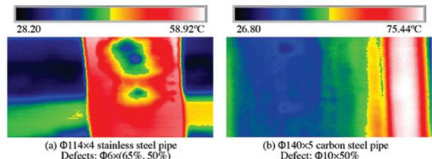
**Figure 6. Thermal images of defects after steam heating and ice cooling**
