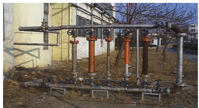
Figure 1. Pressure pipe testing installation for infrared thermography test
