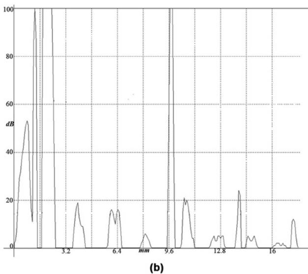
**Figure 4. Ultrasonic A-scan signal display from a non-defective casting having (a) rough surface and (b) machined smooth surface using 10 MHz frequency probe**
