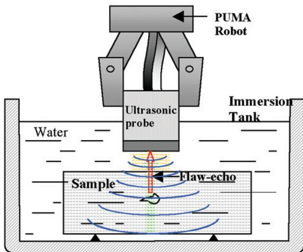
Figure 1. Ultrasonic immersion testing experimental set-up
