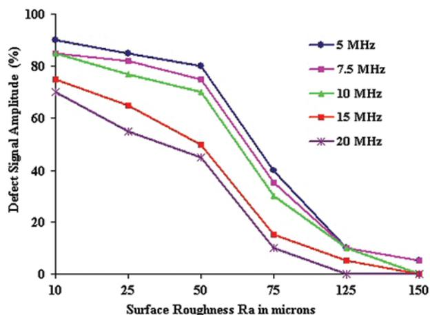
Figure 3. Variation of defect signal amplitude with surface roughness for different frequencies
