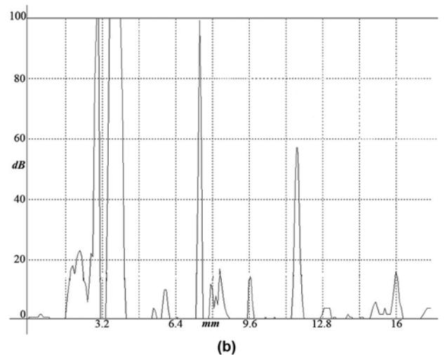
**Figure 5. Ultrasonic A-scan signal display from a defective casting having (a) rough surface and (b) machined smooth surface using 10 MHz frequency probe**
