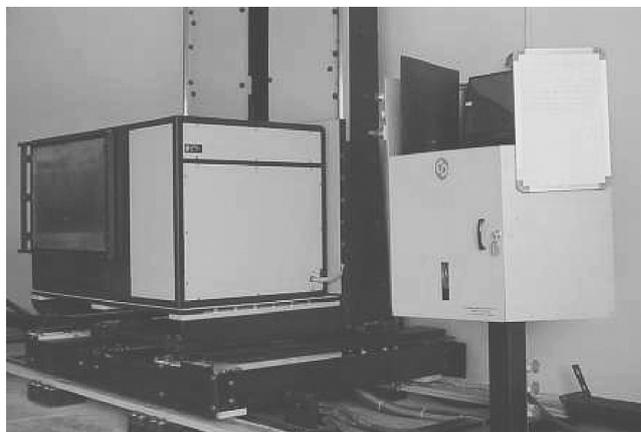
Figure 2. Photograph of digital imaging system for high-energy X-rays
