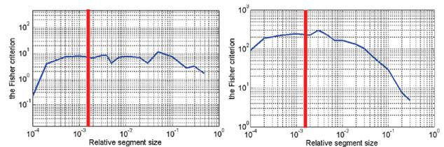
**Figure 1. Values of the Fisher criterion vs the relative segment size for different stiffness ratios: 0.05 (left) and 0.1 (right)**
