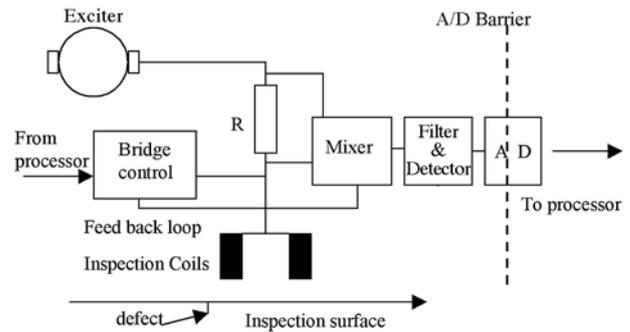
Figure 4. Detector 'B' with added analogue filter to mixer
