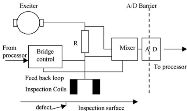
Figure 2. Detector 'A' prototype system
