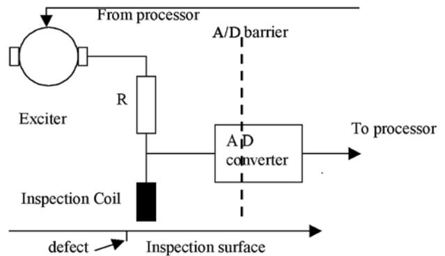
Figure 1. Simple system with A to D barrier forward
