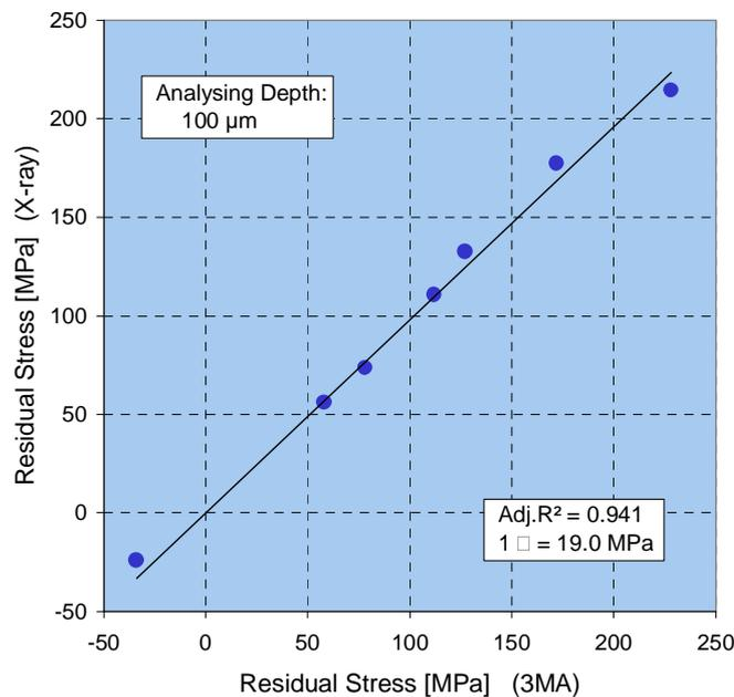
**Figure 10. Residual stress calibration**
