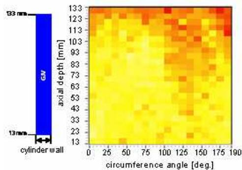
**Figure 7. Coercivity image of a reference block made from GJV**
