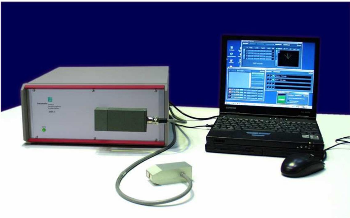
**Figure 1. TCP-IP-based 3MA equipment and software in combination with a laptop**
