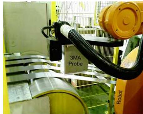
**Figure 3. 3MA with robot at a strip line**
