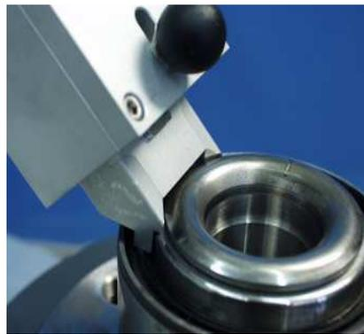
**Figure 9. 3MA-Probe at test location**
