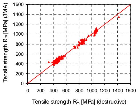
**Figure 4. Tensile strength predicted by 3MA**
