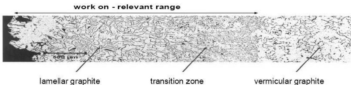
**Figure 5. Microstructure gradient obtained in a cylinder region of a cast engine**
