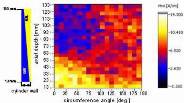
**Figure 8. Coercivity image of block with GJV/GJL gradient**
