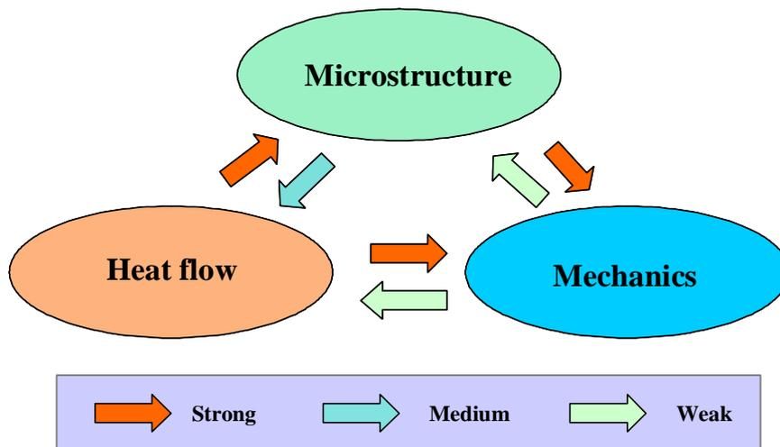
Figure 1. Coupled fields in welding analysis
