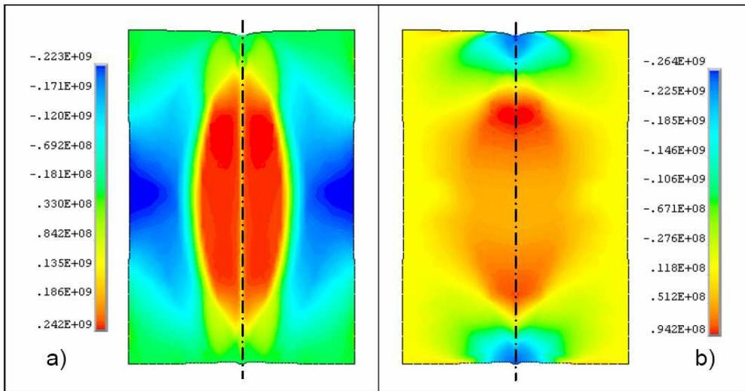
Figure 9. Residual stress distributions (Pa) – Thin plates
