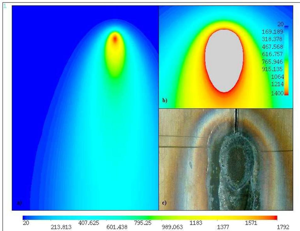
Figure 8. Predicted temperature distribution during thin plates welding
