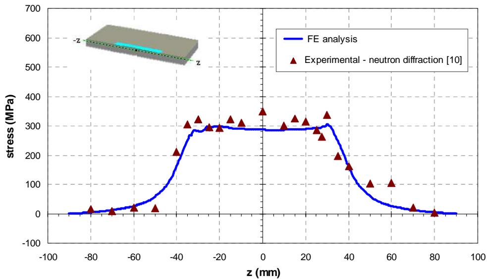
Figure 6. Comparison of predicted and experimentally determined [10] longitudinal stress variation along a longitudinal line, 2 mm beneath the plate top surface
