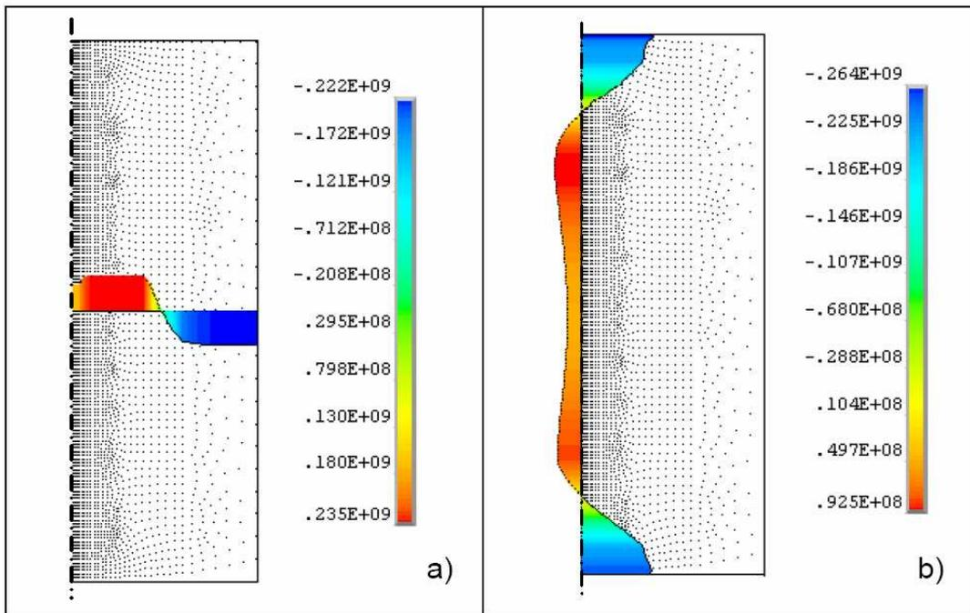
Figure 10. Residual stress (Pa) variation along different lines - Thin plates
