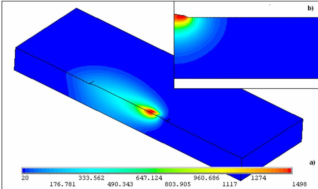
Figure 3. Predicted temperature distribution during welding
