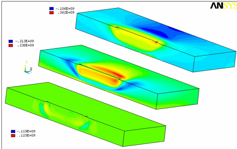
Figure 4. Residual stress distributions (Pa)
