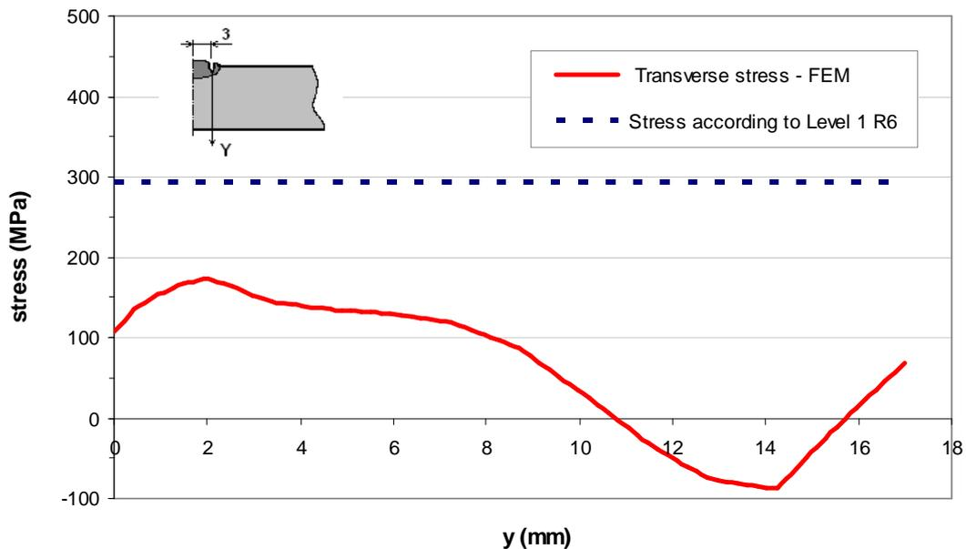
Figure 7. Comparison of predicted residual stress and residual stress quantification according to level 1 of R6 Procedure
