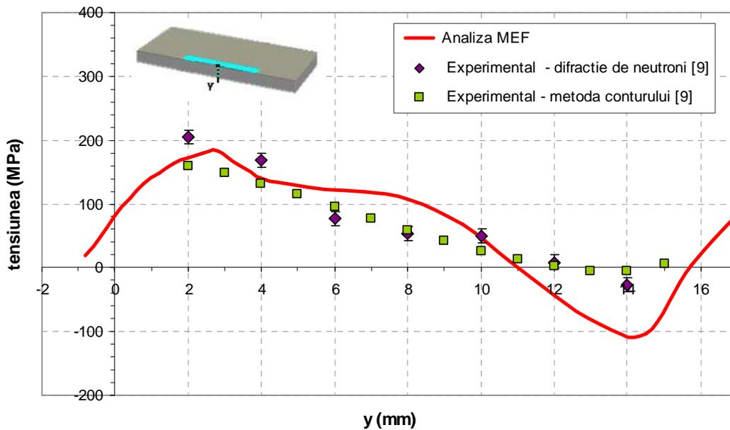
Figure 5. Comparison of predicted and experimentally determined [9] transverse residual stress variation at plate mid, in through-thickness direction
