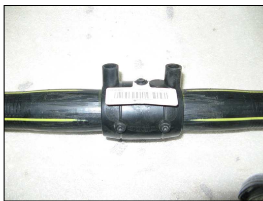
Figure 3. Electrofusion welded joint – socket type
