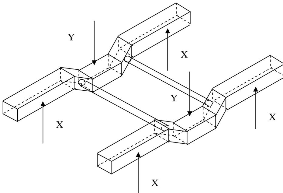
Figure 4. The one piece bogie scheme representation
