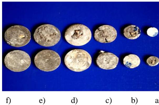
Figure 2. Probes obtained by brazing with neutral flame to carburizing. The marks are: a - 1, b - S1, c - S2, d - S3, e - S4, f - S5 (according to the table 1)
