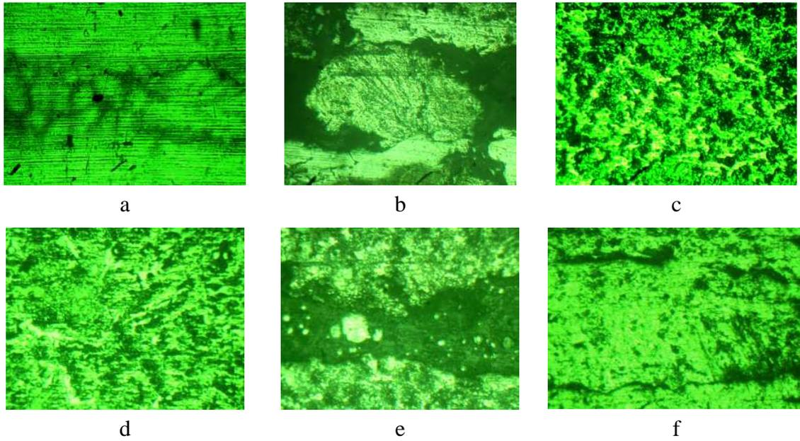
Figure 1. Microstructures of of the joining zones obtained by flame brazing with filler material [100X]
