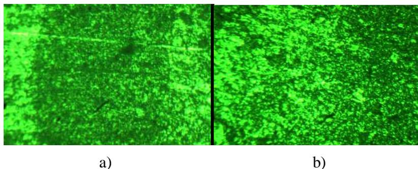
Figure 6. Microstructures of the probes S5 - 3: a -WELD, b -HAZ.
