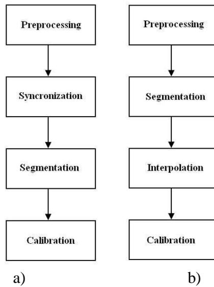
Figure 3. Processing scheme: a) for the rotating probe; b) for the transducer with rotating magnetic field.
