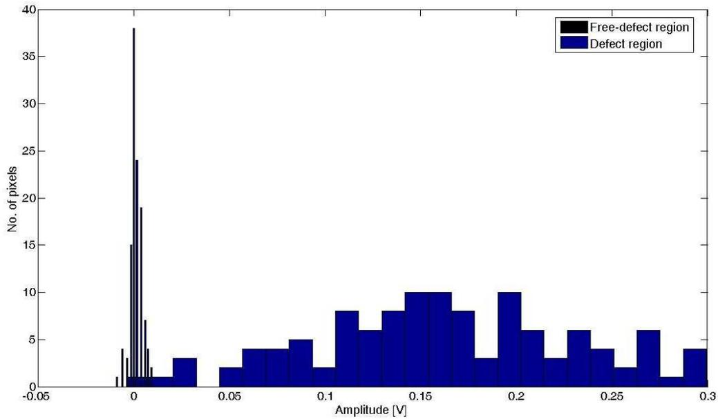
a) Histogram of the amplitude of the signal from the 2 ROI boxes for the imaginary component using the frequency of 100 kHz.
