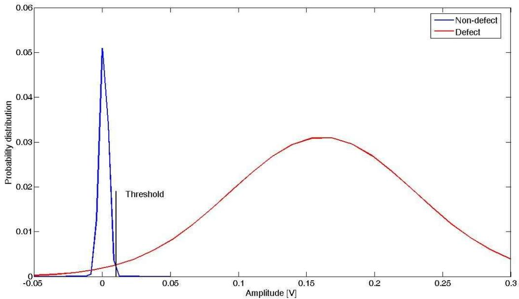
b) The density of probability and choosing of the auto-adaptive threshold defect-non defect, for a probability of false alarm of 5%.
