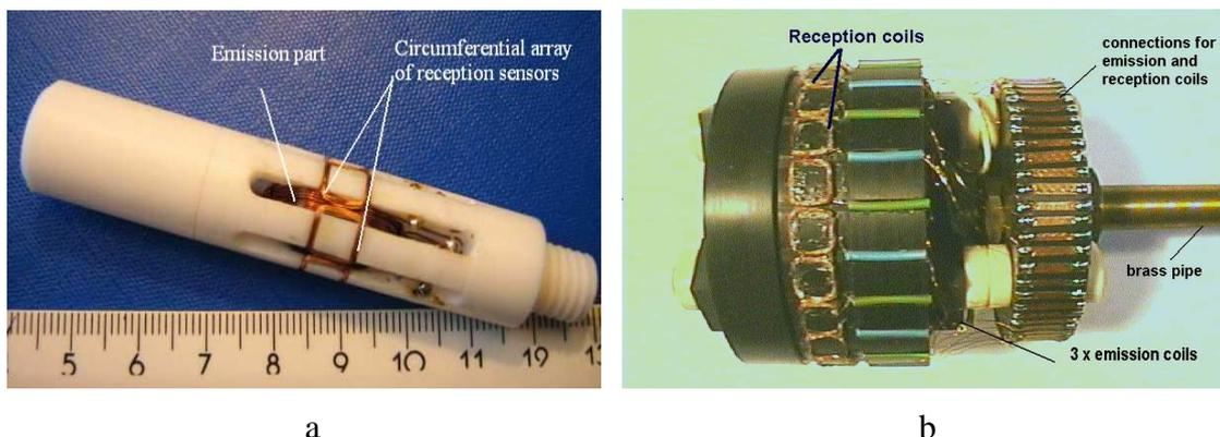
Figure 1. Eddy current inner transducers with rotating magnetic field:
