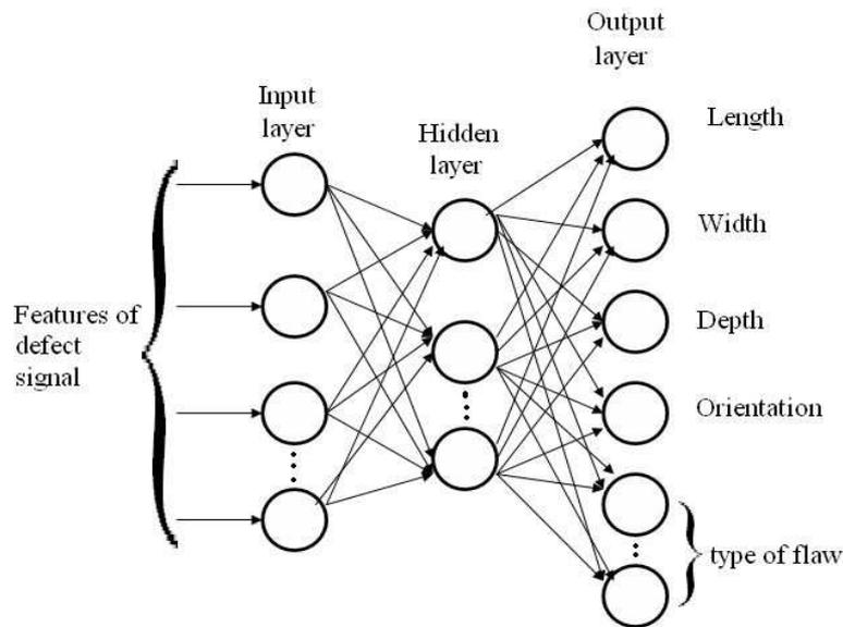
Figure 4. Neural system for automatic data analyses
