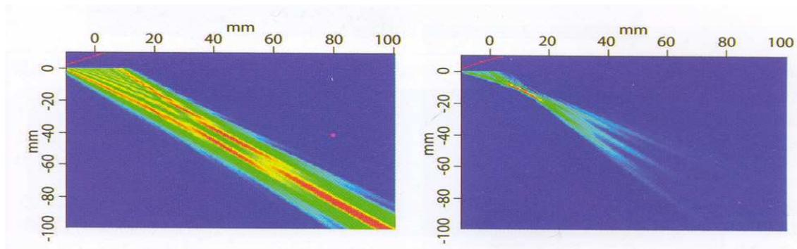
Fig.10. Focus effects modified on beam profiles. *Left*: not focused with natural focal point at 150 mm and beam divergence of 2,4°. *Right*: with electronic focus at 15 mm with beam divergence of 20°.
