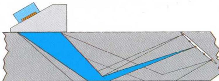
Fig.7. Schematic presentation of the S-Scan inspection of welding. Optimal angles for the middle section are clearly different to the ones for the root's area.
