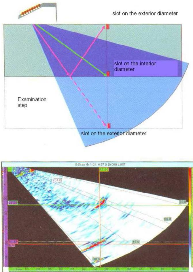
Fig.13. *Up*: an evaluation of the defect localization technique for defects situated at the exterior and interior diameter. *Down*: Resulted S-scan representing the slots
