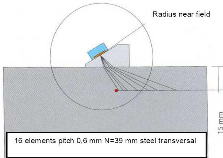
16 elements, 0,6 mm pitch, N=39 mm shear wave in steel
