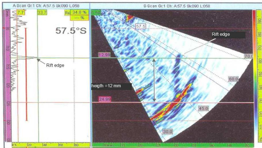
Fig.14. The base and the top of the crack are adequate for a diffusion analysis. A similar approach may be used for cracks on the exterior diameter and for multiple cracks.
