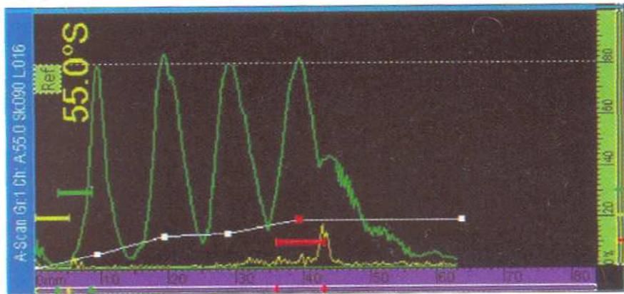
Fig.6. Cylindrical hole scanned using a beam of shear waves at 55°, with calibrated ACG and TCG (low variation of calibration amplitude).
