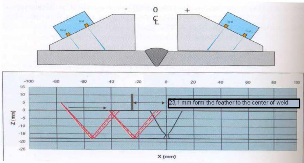
Fig. 11. *Up*: the illustration of the weld inspection using E-Scans
