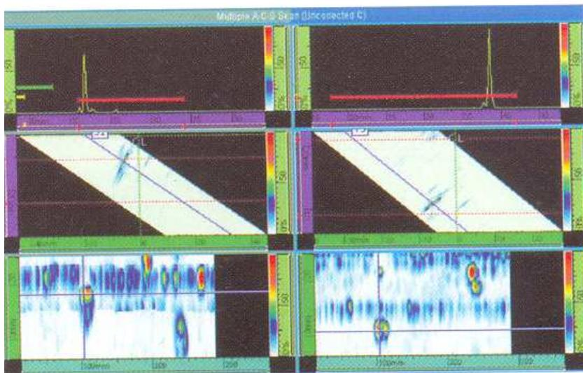
Fig.3. Double E-scan at two different angles on the ultrasonic apparatus, together with A- and C-scans
