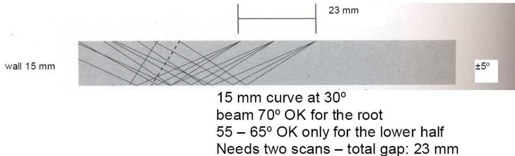
Figure 8 The rays drawing showing the number of the S-Scan passing over requested for a BIA at  $\pm 5^\circ$  to the normal.
