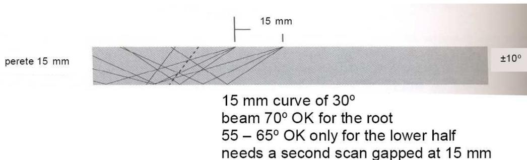
Fig. 9. The rays drawing illustrating the number of the requested S-Scan passings over for a BIA of  $\pm 10^\circ$  to the normal.
