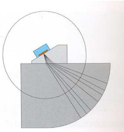
Fig. 5 The calibration on a radius for obtaining an Angle Corrected Gain (ACG).
