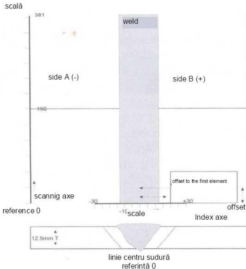
Fig.12. Illustration of the E-Scan procedure, presenting the scan pattern and the distance to the centre of welding.
