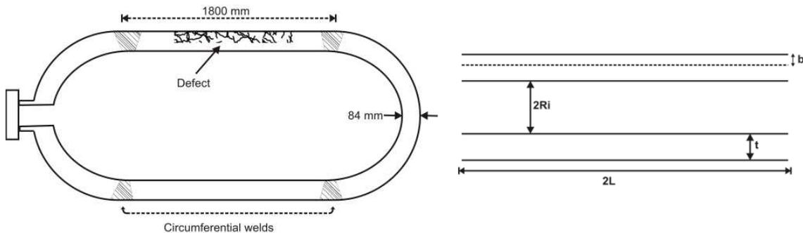
Figure 5. Left: Modified CEBG Test 1 pressure vessel with assumed defect. Right: fracture mechanic crack model used to describe the assumed long external axial surface crack.
