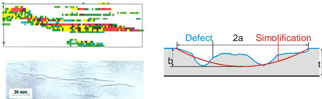
Figure 3. Left: crack detection result in a pipeline from an ultrasonic intelligent pig and corresponding crack pattern in the pipeline. Right: allocation principle of measured crack geometry to model geometry.
