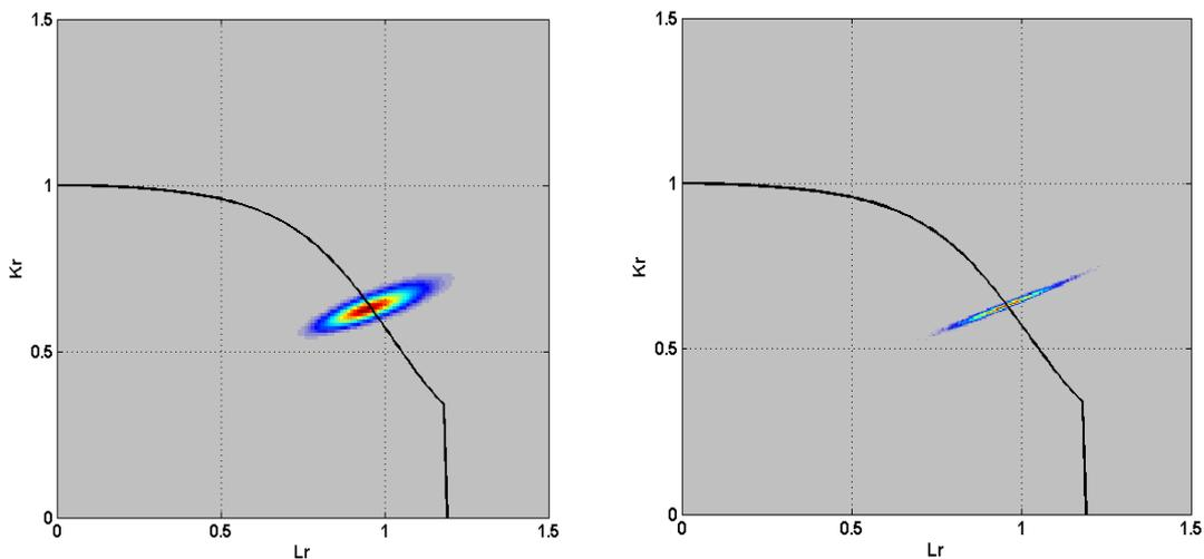
Figure 6. Representation of probability density of probabilistic assessment without considering the POD (left) and with considering the POD information (right). Note that the colour scale is not comparable since the largest value is automatically set to red and the lowest automatically to grey. Therefore, only a qualitative comparison of the visualization of the results is possible.
