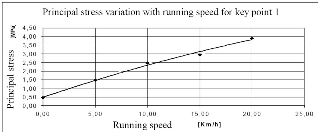
Figure 9. Principal stress variation with running speed for key point 1 (see figure 5).
