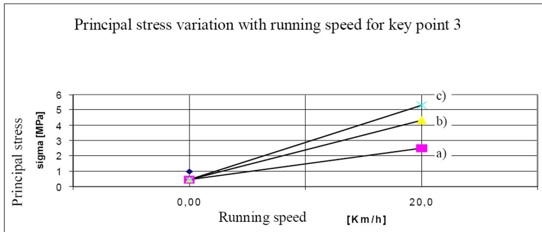
Figure 12. Principal stress  $\sigma_r$  variation with running speed for key point 3 (see figure 5) in comparison with static load of the rail track sample: a) constant running speed of 20 km/h; b) brake procedure with braking shoes from 20 km/h until stop; c) brake procedure with braking shoes and skating pad from 20 km/h until stop.
