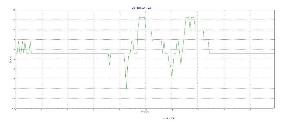
Figure 8. Time variation diagram for the linear specific deformations corresponding to critical area no. 4 of the railtrack sample (measured at 90 mm against the base - Figure 5), for  $v = 10$  km/h running speed value for the tram.
