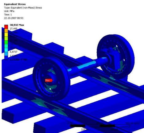
Figure 3. FEA calculus model taking into account the cross-beams supporting the railtrack.
