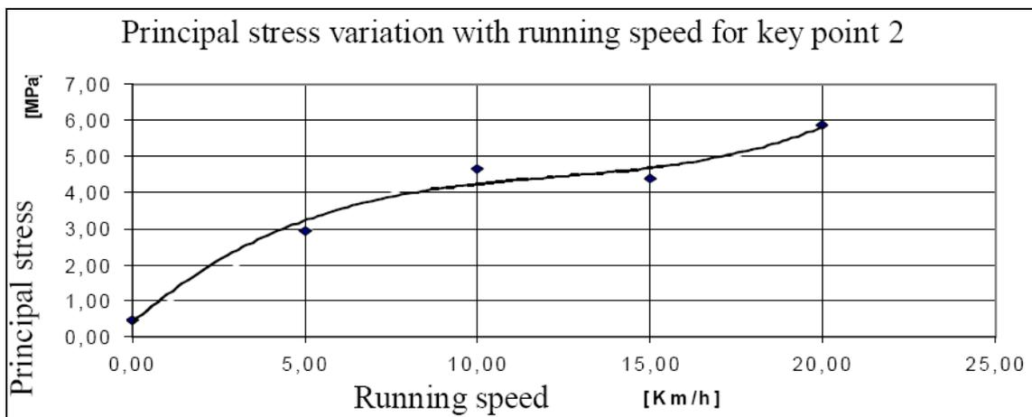
Figure 10. Principal stress variation with running speed for keypoint 2 (see figure 5).
