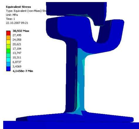
Figure 4. Von Mises stress distribution in FEA calculus model taking into account the cross-beams supporting the rail track.
