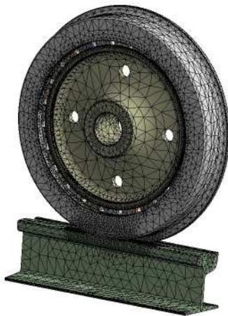
Figure 1. Meshing used in the FEA calculus model.
