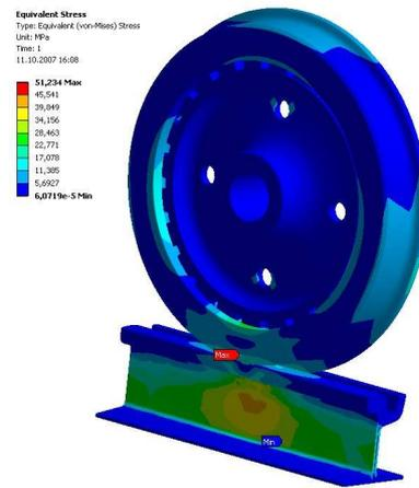
Figure 2. Von Mises stress distribution.
