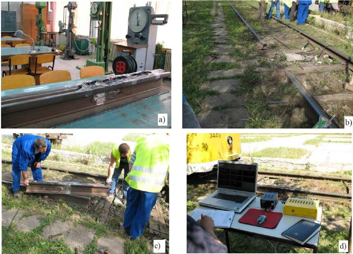
Figure 7. Experimental measurements of the stress-strain state of the wheel-rail track assembly through resistive electric gage principle: a) rail track sample with bonded resistive strain gauges; b), c) positioning of the rail track sample in a railway route for measurements of the stress-strain state at the wheel-rail track assembly; d) overall picture above the in-site experimental measurements.
