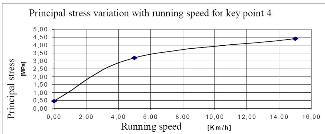
Figure 11. Principal stress variation with running speed for keypoint 4 (see figure 5).
