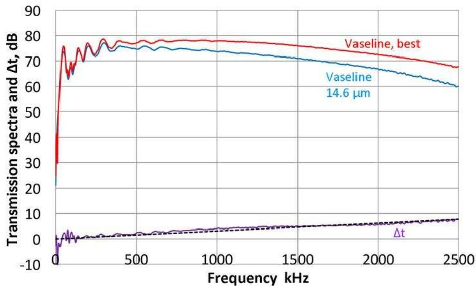
Fig. 6 Transmission spectra,  $t$ , of received signals through Vaseline couplant. Vaseline reference: red curve, Vaseline couplant after normal mounting: blue. Spectral difference,  $\Delta t$ , between normal and reference installation is plotted in purple curve, which follows linear frequency dependence in black dash line.  $\Delta t$  (dB) = 3.10  $f$  (MHz). FC500 transmitter and Olympus V104 receiver.
