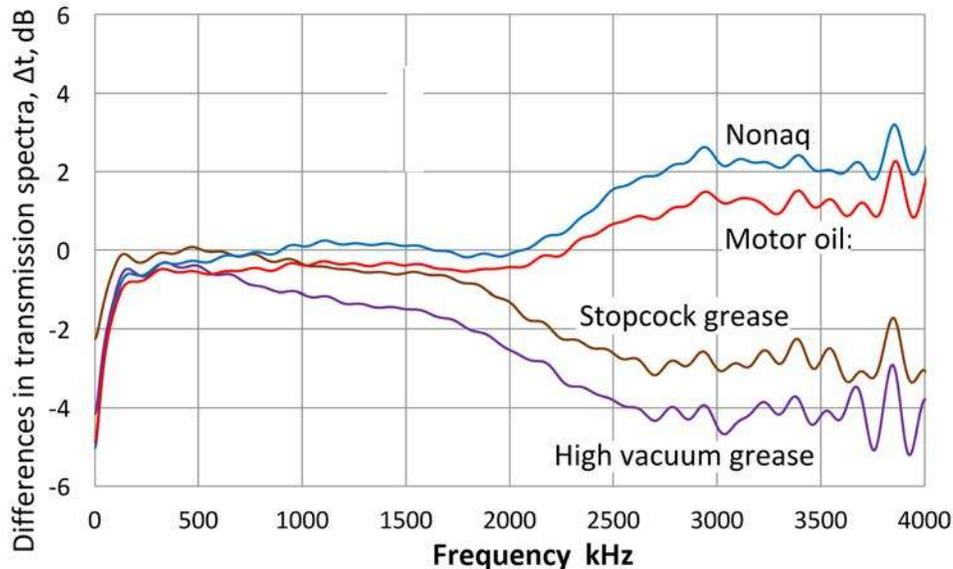
Fig. 3 Differences in transmission spectra,  $\Delta t$ , of received signals through couplant using Vaseline spectrum as reference up to 4 MHz. Motor oil: red, Nonaq: blue, High vacuum grease: purple, Stopcock grease: brown. NDT Systems C16 transmitter and FC500 receiver.
