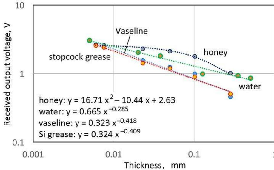
Fig. 7 Thickness dependence of output voltage of received signals through honey (dark blue), water (green), Vaseline (blue), stopcock grease (red). FC500 transmitter and Olympus V104 receiver.
