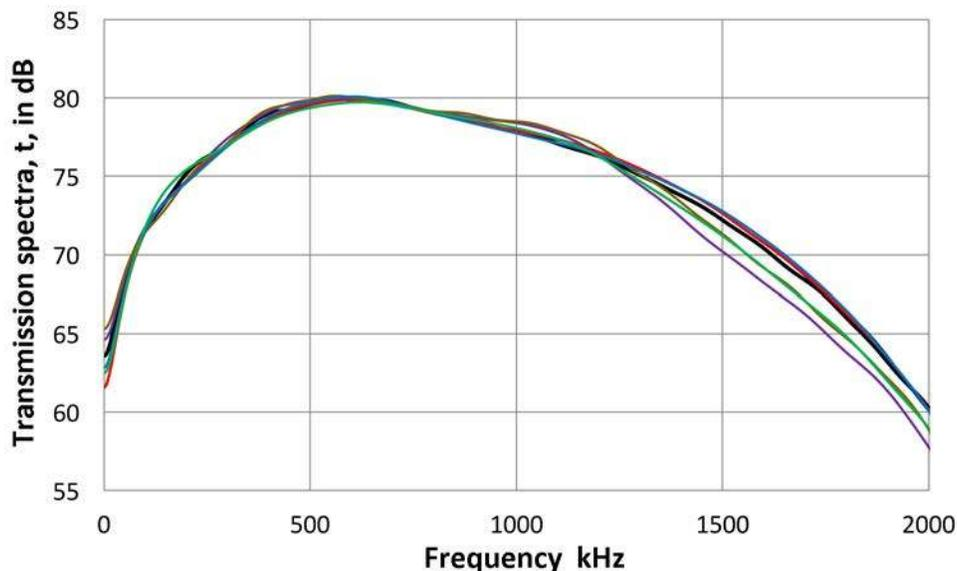
Fig. 1 FFT magnitude spectra of received signals through couplant, or  $t$  vs. frequency,  $f$ . Vaseline: dark blue curve, motor oil: red, Nonaq: blue, High vacuum grease: purple, Stopcock grease: brown, SC-6 resin: green. V103 transmitter and FC500 receiver.
