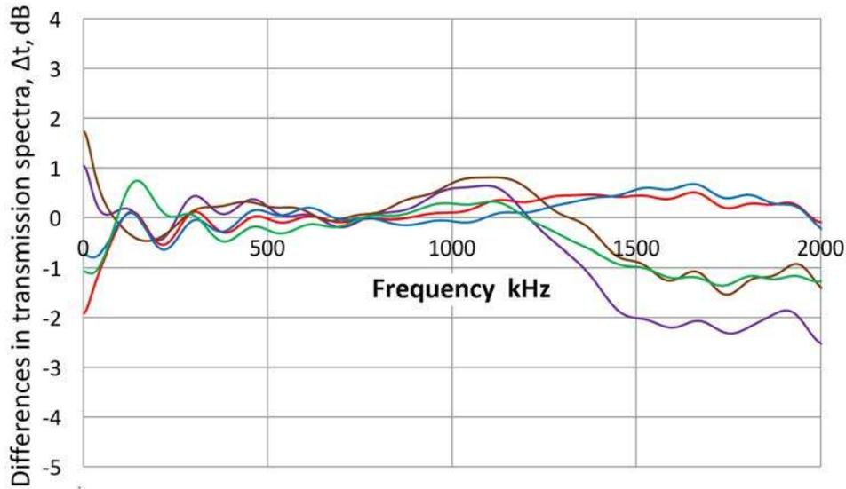
Fig. 2 Differences in transmission spectra,  $\Delta t$ , of received signals through couplant using Vaseline spectrum as reference. Motor oil: red, Nonaq: blue, High vacuum grease: purple, Stopcock grease: brown, SC-6 resin: green. V103 transmitter and FC500 receiver.
