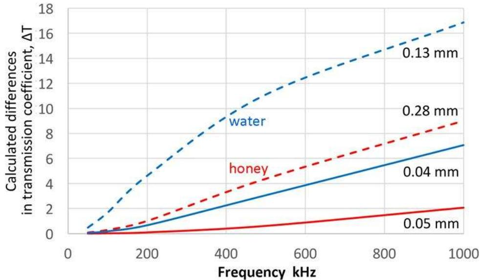
Fig. 10 Calculated differences in transmission coefficient,  $\Delta T$ , through a gap filled with water and honey vs. frequency. Water thickness = 0.04 mm (blue curve), 0.13 mm (blue dash); honey thickness = 0.05 mm (red), 0.28 mm (red dash).
