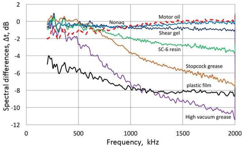
Fig. 4 Differences in transmission spectra of received signals,  $\Delta t$ , through couplant using Vaseline spectrum as reference. Non-optimum sensor installation for viscous couplants. Motor oil: red, Nonaq: blue, Shear gel: dark blue, High vacuum grease: purple, Stopcock grease: brown, SC-6 resin: green, plastic film: black. V103 transmitter and FC500 receiver.
