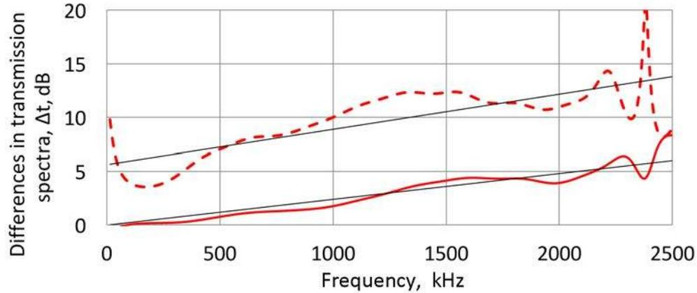
Fig. 8b Spectral difference,  $\Delta t$ , between reference installation and through 0.05 mm (solid) and 0.28 mm (dashed) layer of honey.  $\Delta t$  curves follow nearly linear frequency dependence in black lines without offset (0.05 mm) or with offset (0.28 mm). FC500 transmitter and Olympus V104 receiver.
