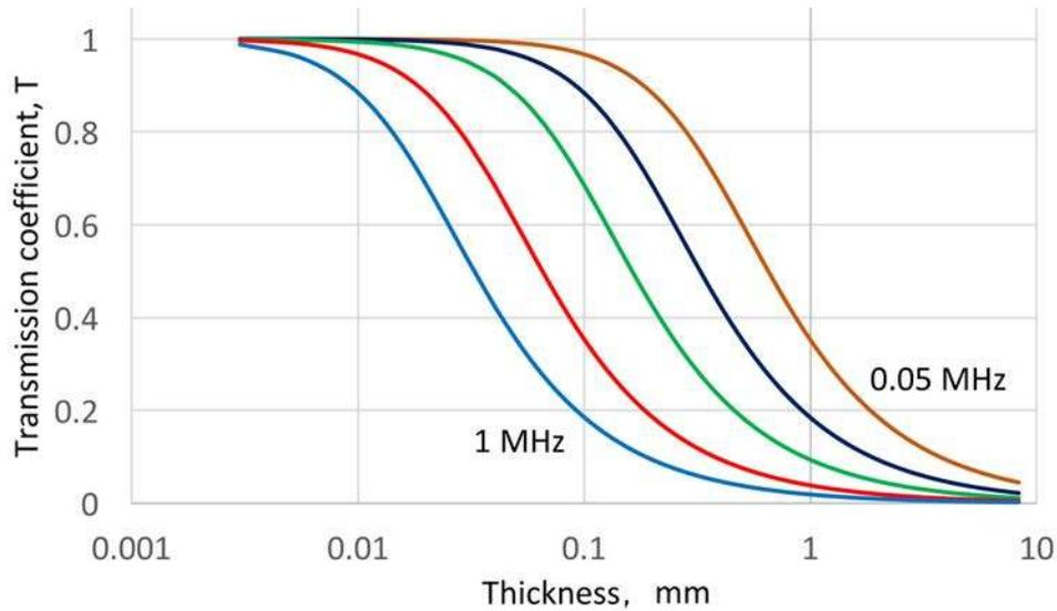
Fig. 9a Transmission coefficient, T, through a gap filled with water vs. gap thickness.  $f = 1$  MHz (blue curve), 0.5 MHz (red), 0.2 MHz (green), 0.1 MHz (dark blue) and 0.05 MHz (brown).
