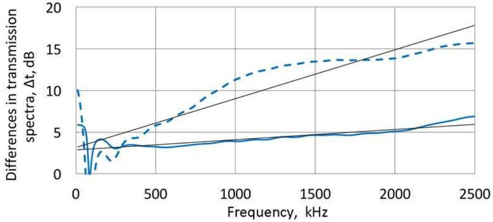
Fig. 8a Spectral difference,  $\Delta t$ , between reference installation and through 0.04 mm (solid) and 0.13 mm (dashed) layer of water.  $\Delta t$  curves follow nearly linear frequency dependence in black lines with offset. FC500 transmitter and Olympus V104 receiver.
