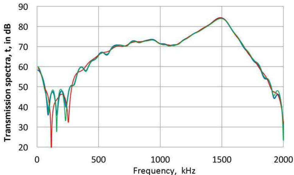
Fig. 5 Transmission spectra,  $t$ , of received signals through couplant. Vaseline reference: blue curve, epoxy resin (as mixed): green, epoxy resin (cured for 30 min): red. FC500 transmitter and Automation Ind. 1 MHz-1/2".
