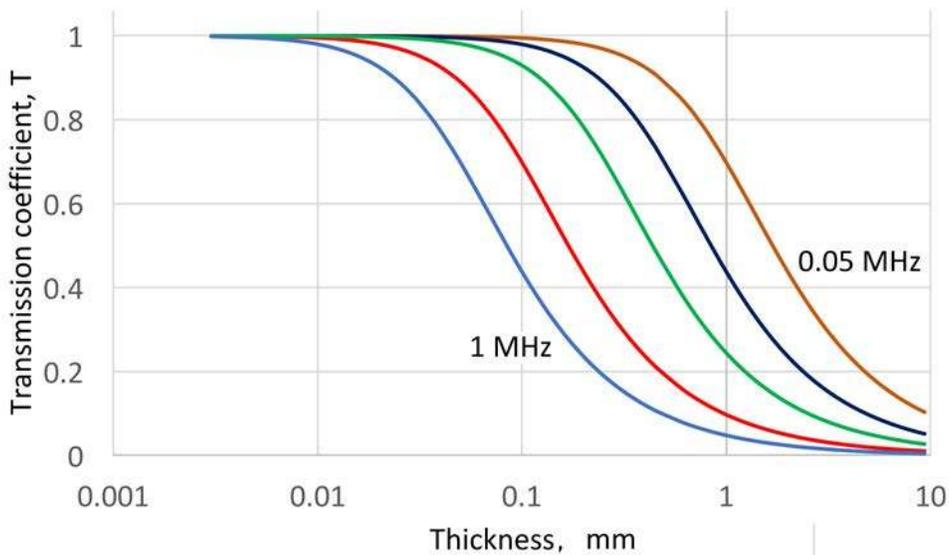
Fig. 9b Transmission coefficient, T, through a gap filled with honey vs. gap thickness.  $f = 1$  MHz (blue curve), 0.5 MHz (red), 0.2 MHz (green), 0.1 MHz (dark blue) and 0.05 MHz (brown).
