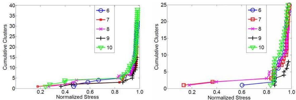
Fig. 5. Cumulative cluster growth for cross-ply specimen: sensors 1 (left) and 2 (right). Cluster sizes of 6 to 10 were plotted. This behavior was seen for quasi-specimens as well (not shown).
