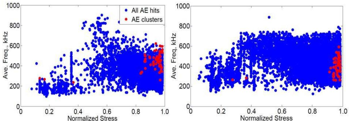
Fig 7. Average frequency of cluster signals (red) and all AE data measured in cross-ply specimen: data from sensor near failure (left), away from failure (right).
