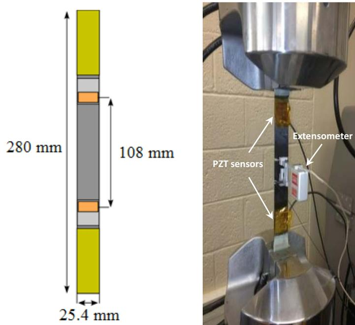
Fig. 1. Tensile specimen dimensions (left) showing dimensions of the length and sensor to sensor distance, specimen during testing.
