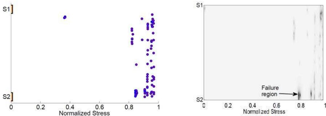
Fig. 9. Raw AE cluster location for clusters of 10 (left) seen in cross-ply specimen. Right figure shows the cluster location data transformed into a cluster density plot to highlight the location of clusters.
