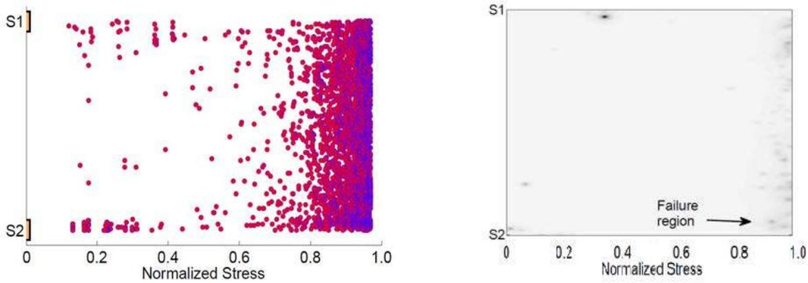
Fig. 8. Raw AE location data for unclustered data (left) and signal density of the unclustered data (right) plots for cross-ply specimen. S1 and S2 refer to sensors 1 & 2, which were 75 mm apart. Events are the individual dots. The black area in right plot is due to dense AE activity.
