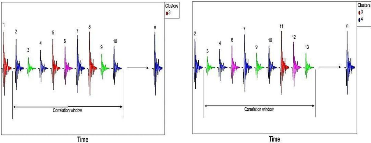
Fig. 2. Schematic of clustering process with like signals colored the same. Numbers correspond to the order that the signals were detected.
