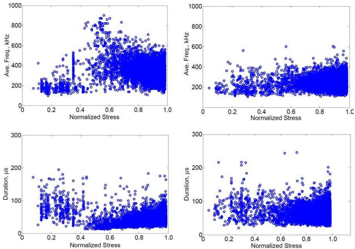
Fig. 4. Typical average frequency and duration plots seen for the two different lay-ups: cross-ply (left), quasi-isotropic (right).
