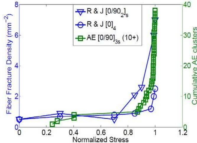
Fig. 6. Comparison of AE clusters seen in cross-ply to fiber break measurements using SEM [1].
