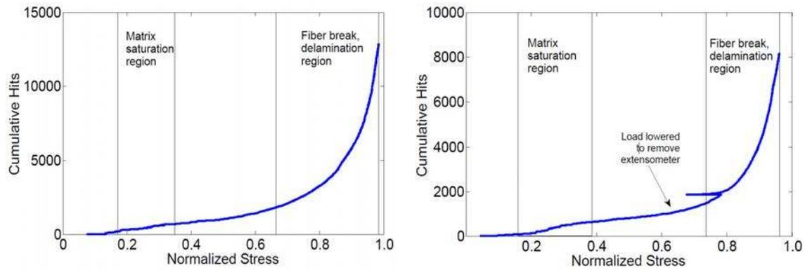
Fig. 3. Cumulative AE hits vs stress for cross-ply (left) and quasi-isotropic (right).
