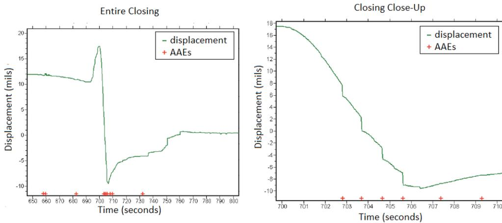
Figure 7: Correlation of AAEs with displacement along the interface between the bascule girder bottom flange and the curved upper track plate during bridge closing, showing (a) entire closing and (b) close-up of 10 second period of greatest movement
