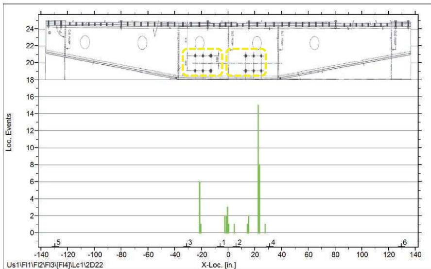
Figure 11: Distribution of AAE source locations along pinion girder. Pinion bearing/box girder through-bolt groups are highlighted in yellow. Figure courtesy of Daniel Marron (unpublished data).
