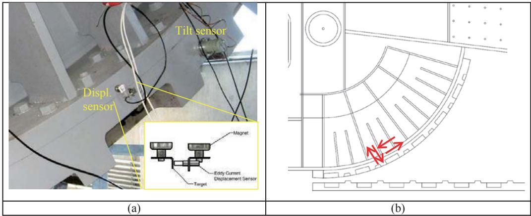
Figure 6: Photograph and sketch showing displacement sensor (a) location and (b) orientation (exaggerated scale) on bascule girder - upper track plate interface
