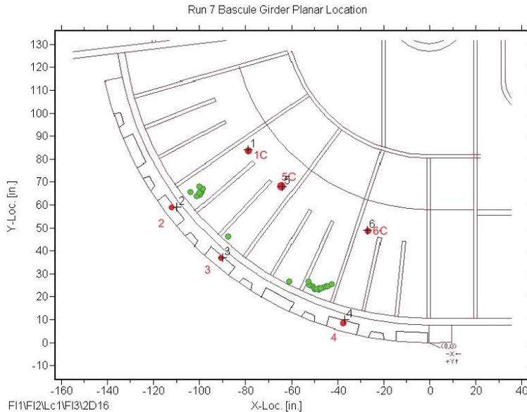
Figure 5: Planar location results showing events along bottom flange of bascule girder heel. AE transducer locations are indicated by the numbered red dots, and located AE events by green dots.
