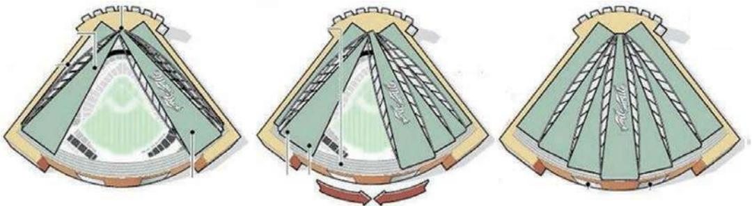
Figure 1: Stadium roof closing sequence showing roof panels pivoting on bearings above home plate (*Milwaukee Journal-Sentinel* illustration)
