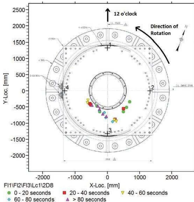
Figure 9: Arc of located events (divided into 20-second time bins) in pivot area during rotation of swing bridge
