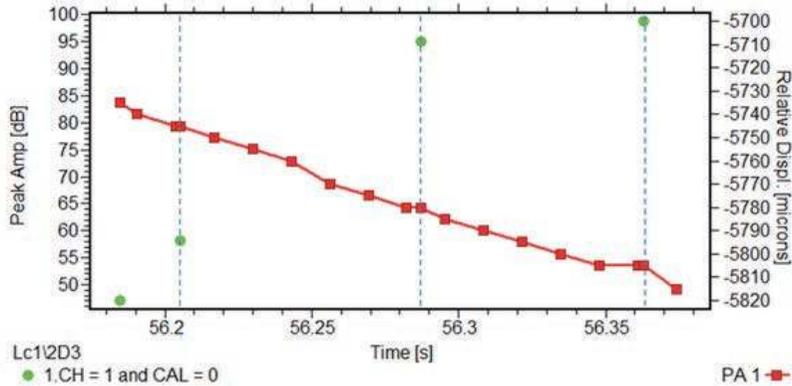
Figure 3: Time history of AE amplitude (green dots) and roof panel truss displacement (red line) showing correlation between AE and changes in displacement rate. Dashed lines indicate times of AE events, for comparison to displacement data.
