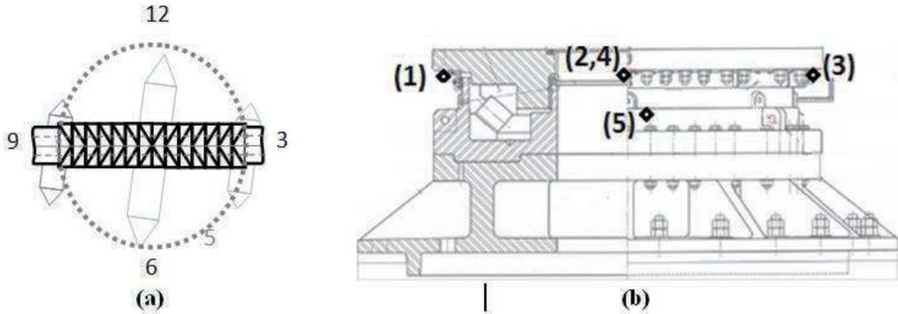
Figure 8: (a) Plan view of swing bridge with clock face representation of bridge angle superimposed; (b) Elevation view of sketch of AE transducer layout on pivot
