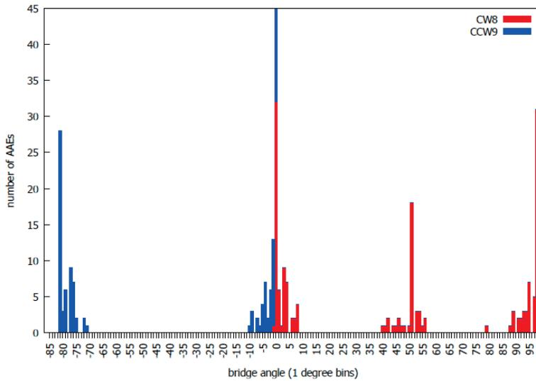
Figure 10: Stacked histogram of AAEs (n = 257) with bridge angle for selected clockwise (red) and counterclockwise (blue) bridge movements, showing clusters of AAEs at starts and stops, including a pause at +52 degrees during clockwise motion. Figure courtesy of Daniel Marron (unpublished data).
