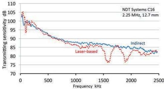
Fig. 5  $T_{NDT}$  by laser-based and indirect methods.
