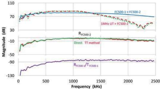
Fig. 12 Spectra for  $R_{FC500-2}$  with a tri-transducer test.
