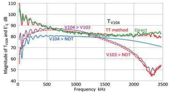
Fig. 13  $T_{V104}$  by direct (laser) and TT methods.
