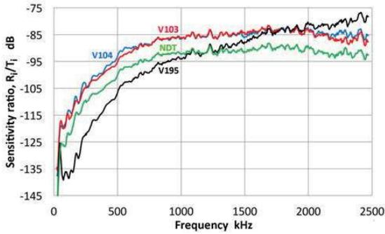
Fig. 10 Spectral ratio,  $R_i/T_i$ , for four transducers.
