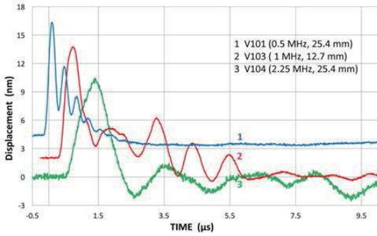
Fig. 1 a. Displacement waveforms of three transducers.
