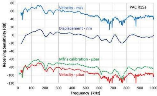
Fig. 9 Velocity calibration curves of R15a sensor.
