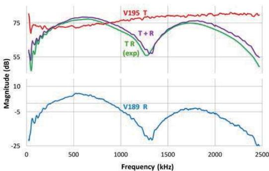
Fig. 7 Combined  $T_{V195} + R_{V189}$  vs. TR test spectrum.
