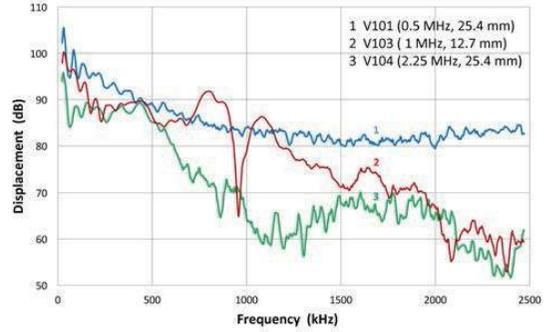
b. FFT displacement spectra, re. 0 dB at 1 nm.
