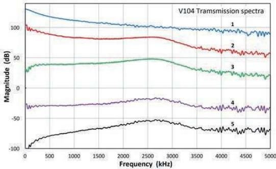
Once  $T_{V104}$  of the reference transducer is obtained, we determine  $R_i$  of other transducers by conducting T-R test in a face-to-face arrangement of the reference against a sensor under test (SUT) using equation (1). This provides  $E^\circ$  for the transducer-sensor pair. The  $R_{SUT}$  is then determined by  $R_{SUT} = E^\circ - T_{V104}$ . The 0 dB reference for the  $R_{SUT}$  is 1 V/nm with frequency in kHz.
