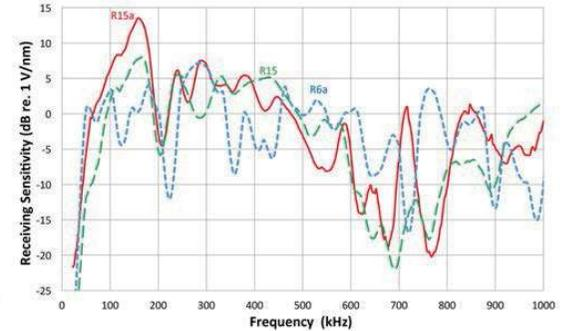
Fig. 4 Receiving sensitivities of 3 AE sensors.
