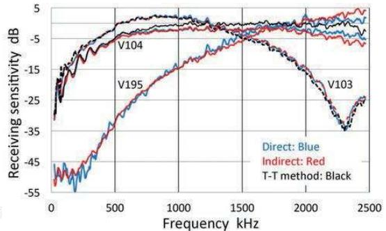
Fig. 6  $R_i$  spectra of 3 transducers by various methods.
