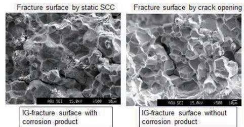
Figure 3: SEM of fracture surfaces by the static SCC test (the left) and by the crack opening operation of the sensitized type-304 (650°C x 90min) by 1% tetra-thionic acid (pH=2)
