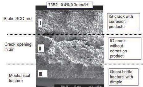
Figure 13: SEM of fracture surface of the brass attacked by 8% ammonia vapor and then crack opening operation in air
