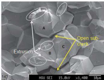
Figure 7: SEM of the fracture surface produced by the crack opening operation in air of the type-304 strip previously SCC tested in 1% tetra-thionic acid
