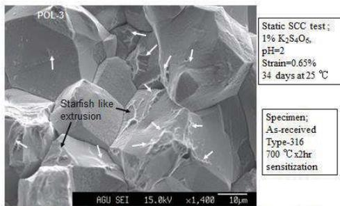
Figure 10: SEM of the fracture surface produced by crack opening operation in air of the sensitized type-316 steel previously suffered IG-SCC by static SCC test
