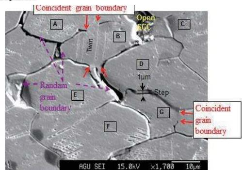
Figure 5: SEM of the free surface of type-304 strip with IG-SCC after the crack opening operation in air
