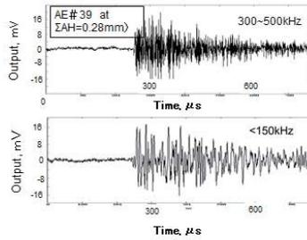
Figure15 : Waveform and frequency components spectrum of AE during crack opening operation of the 70/30 brass previously attacked by 8% ammonia
