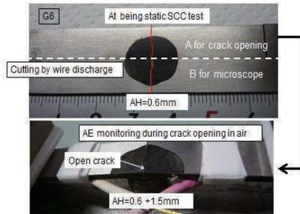
Figure 1: specimen with IG-SCC by static three point bending (the upper) and AE monitoring method during the crack opening of the longitudinally cut specimen
