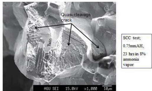
Figure 17: SEM of the fracture surface by crack opening operation of the brass previously attacked by 8% ammonia vapor
