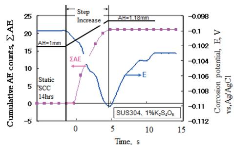
Figure 9: Change of AE and corrosion potential of the sensitized Type-304 steel during the static SCC test and step-wise load increase in the tetra-thionic solution
