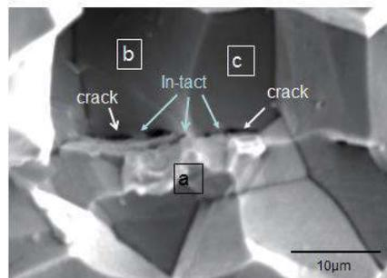
Figure 8: SEM of the fracture surface produced by crack opening operation of the type-304 strip previously SCC tested in 1% tetra-thionic acid.
