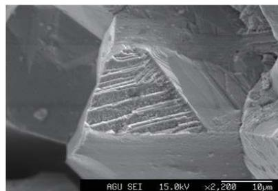
Figure 18 :SEM of the fracture surface by crack opening operation in air after the static SCC test
