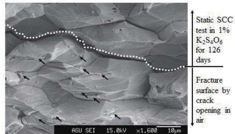
Figure 11: SEM of the fracture surface produced by crack opening operation in air of the 35% cold rolled and then sensitized ( $700\text{ }^{\circ}\text{C} \times 2\text{ hrs}$ ) type-316 steel
