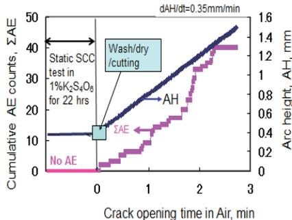
Figure 4: Acoustic emission during the static SCC test and the crack opening operation of the type-304 steel strip
