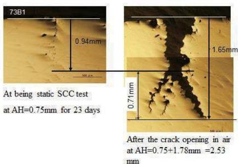
Figure 12: Transverse IG-SCC of 70/30 brass by 8% ammonia vapor.
