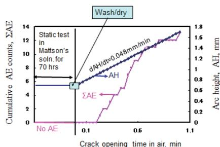
Figure 19: Acoustic emission during the static SCC test and crack opening in air of 70/30 brass previously attacked by Mattson's solution
