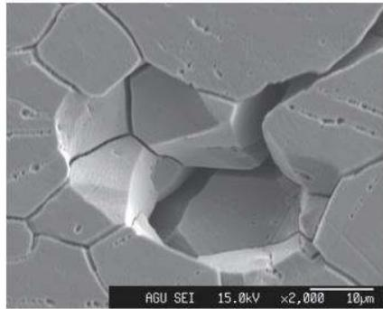
Figure 6: Falling-off of grains in sensitized type-304 steel by the corrosion of random grain boundaries
