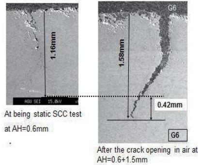
Figure 2: transverse IG-SCC of sensitized (650°C x 90min) type-304 steel by 1% tetra-thionic acid (pH=2).
