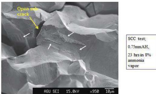
Figure 16 :SEM of the fracture surface produced by crack opening operation of the brass previously attacked by 8% ammonia vapor
