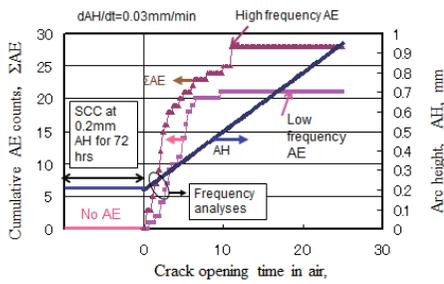
Figure 14 :Acoustic emission during static SCC test and crack opening in air of 70/30 brass previously attacked by 8% ammonia vapor
