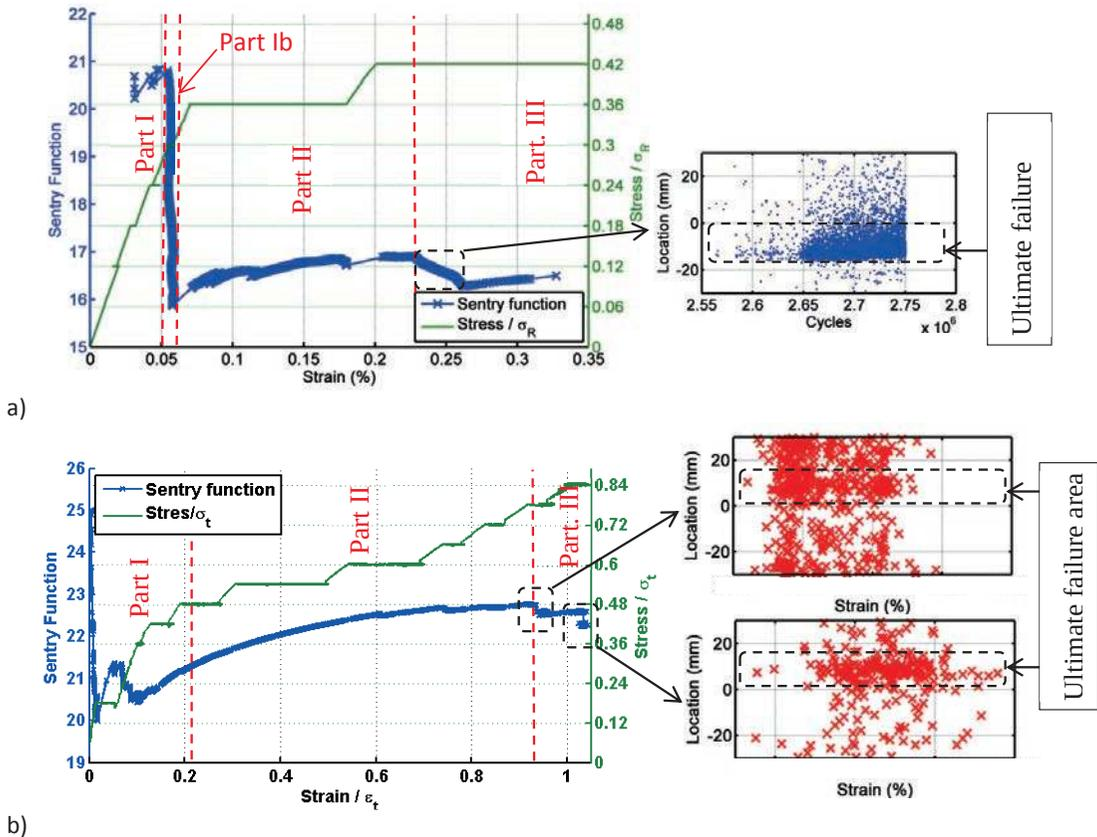
Figure 2 : Coupling of mechanical energy and acoustic energy (Sentry function) for a) an incremental cyclic fatigue test and b) an incremental static fatigue test
