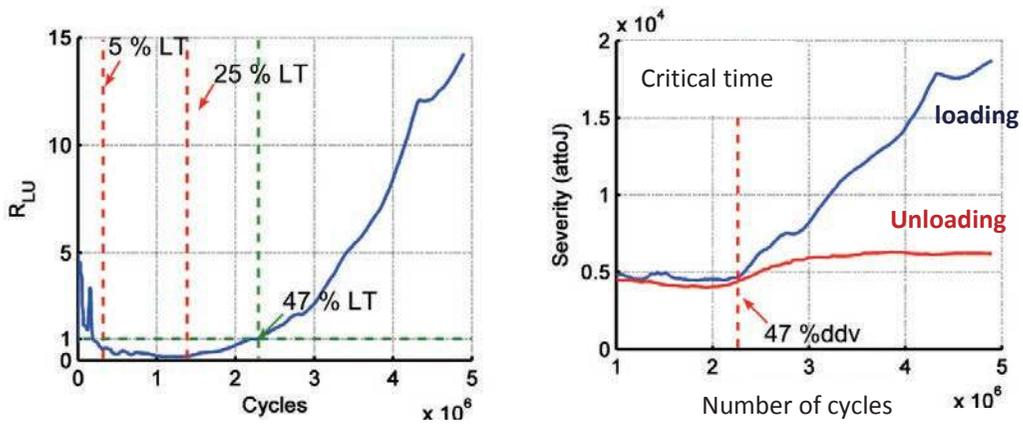
Figure 4: a) Evolution of the coefficient  $R_{LU}$  during cyclic fatigue at constant amplitude and highlight of two characteristic times at 25 % and 47 % of the lifetime duration (LT lifetime) on  $SiC_f/[Si-B-C]$  composites, b) Evolution of the severity
