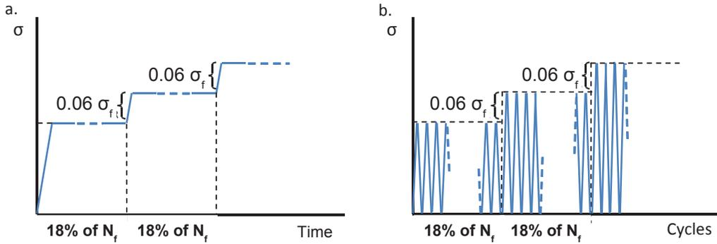
Figure 1. Applied stress for a. Incremental static fatigue test b. Incremental cyclic fatigue test
