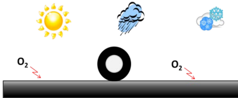
Fig. 1. Oxidative aging of asphalt concrete pavements. With increasing oxidative aging in the top material layer, the pavement becomes increasingly more susceptible to damage accumulation due to mechanical and environmental loads.
