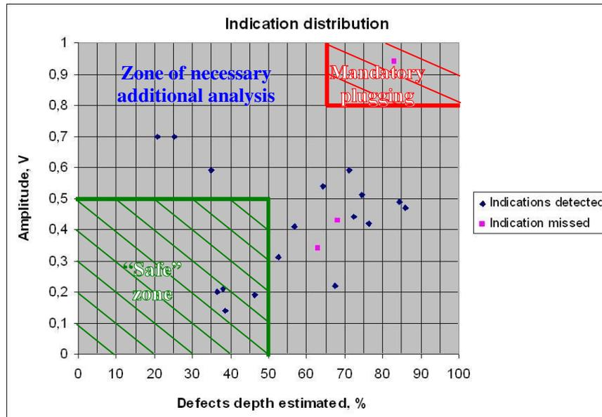
Figure 2 - Distribution of defects in different zones indicated in plugging criteria according to defect parameters (depth estimated according to ET results and amplitude)
