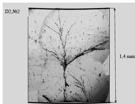
Fig. 1 - Results of metallography study. Defect depth: 100%. Extension: 7 mm
