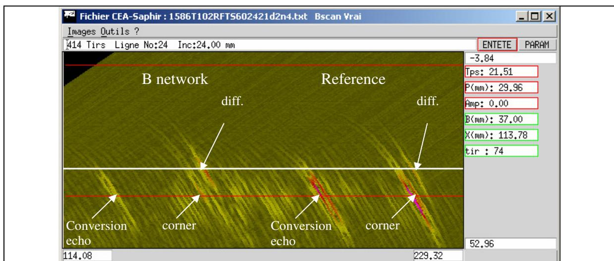
Figure 5 - LW60°-2 MHz probe
