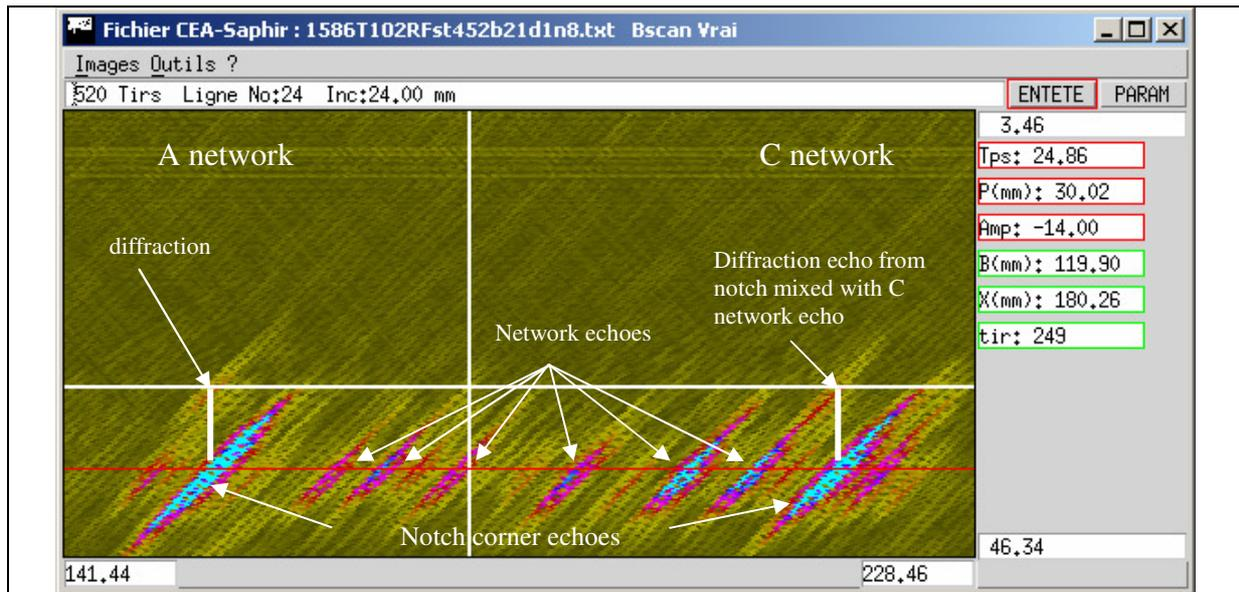
Figure 3 - SW45°-2 MHz probe (component internal wall in red, notches in white and white cursor at the top of the notches)
