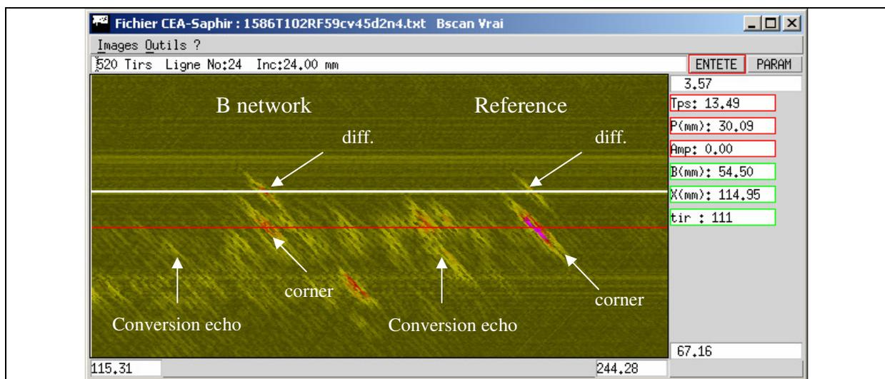
Figure 4 - LW45°-2 MHz probe
