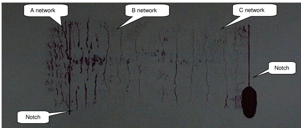
Figure 1 - Dye penetrant test of the cracked mock-up in the presence of the electro-eroded notches
