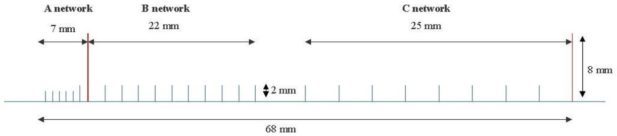
Figure 2 - Schematic representation of the three networks obtained (blue) and of the two notches (red)
