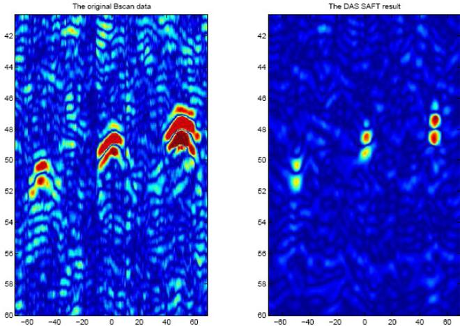
Figure 5 – B-scans of the 3 holes in the SS cube in contact mode. Raw data (left) and the result of SAFT processing (right).
