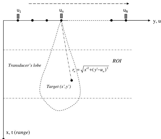
Figure 1 – 2D geometry appropriate for broadside strip-map mode synthetic aperture.
