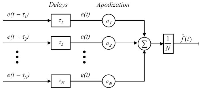
Figure 2 – Block diagram for the delay-and-sum SAFT system. DAS generates a sum of delayed signals received at different transducer positions. Each signal can also be multiplied by the apodization coefficient to reduce the side lobes in the resulting beampattern.
