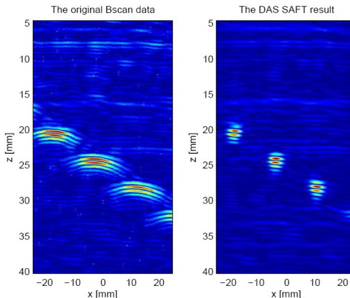
Figure 7 – B-scans of the 4 holes in the copper block in immersion mode. Raw data (left) and the result of SAFT processing (right).
