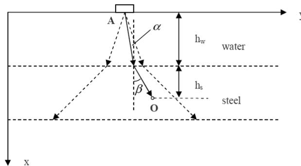
Figure 3 - Beam refraction in the immersion mode – the ultrasonic wave chooses the path between two points which takes the least time.
