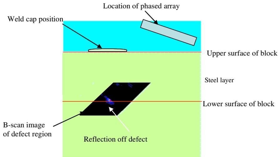
Figure 10 - Experimental results obtained for inspection of Defect 1 with a wedge coupled phased array using a 20 element transducer aperture.
