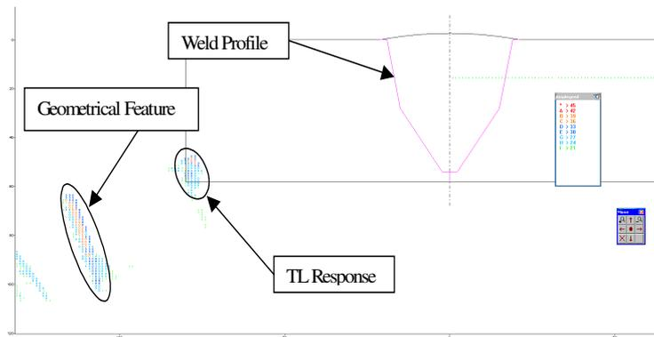
Figure 13 - Experimental results for inspection of Defect 2 with a single crystal transducer.
