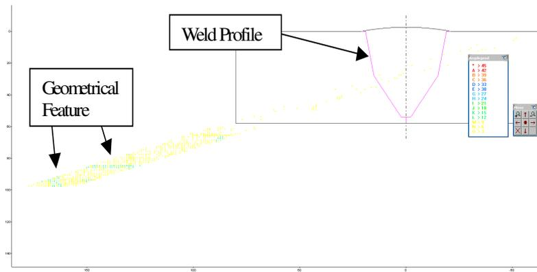
Figure 15 - Experimental results obtained for inspection of Defect 3 with a single crystal transducer.
