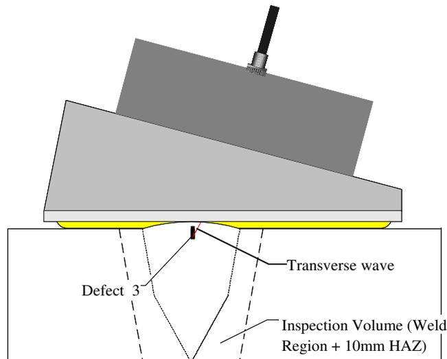
Figure 8 - Experimental set-up to demonstrate the capability for near surface inspection in region of a weld cap using the membrane coupled phased array device.
