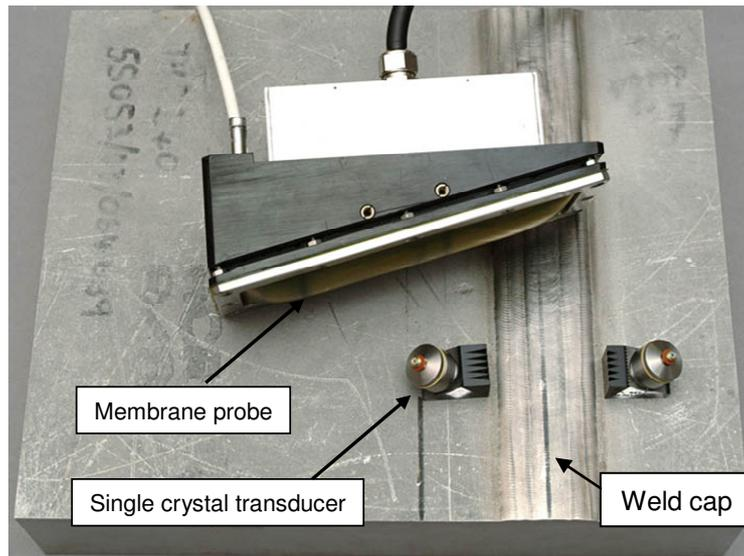
Figure 1 - Photograph of membrane coupled conformable phased array device seen along with conventional single crystal transducers and stainless steel test piece.
