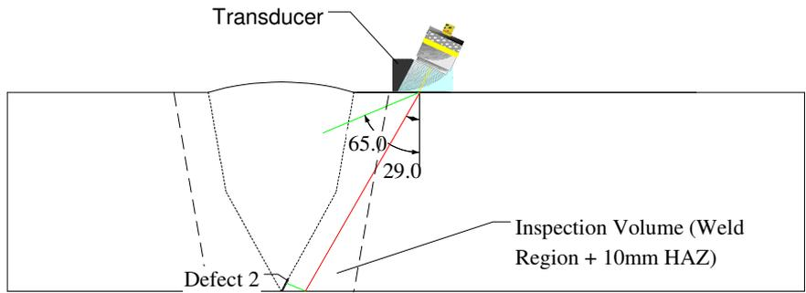
Figure 5 - Schematic of pulse-echo Transverse-Longitudinal mode conversion inspection of Defect 2 (lack of fusion in side wall) using a single crystal transducer.
