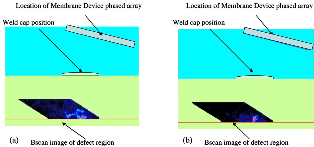
Figure 12 - Experimental results for inspection of Defect 2 (lack of sidewall fusion in root region) using membrane device in pulse echo mode using shear waves mode-converted at block lower surface. (a) plane surface delay laws applied; (b) updated delay laws applied.
