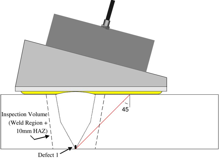
Figure 4 - Schematic of pulse-echo shear wave inspection technique of Defect 1 using the membrane coupled phased array device.
