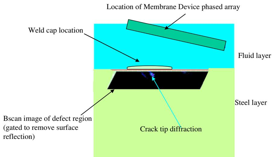
Figure 14 0 Experimental results using membrane device showing B-scan image of Defect 3 obtained using a 15 element transducer aperture.
