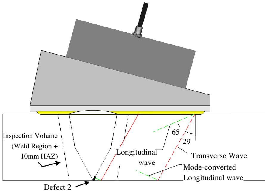
Figure 6 - Schematic of pulse echo Transverse-Longitudinal mode conversion inspection of Defect 2 using the membrane coupled phased array device.
