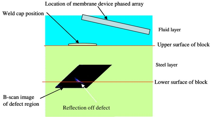
Figure 9 - Experimental results obtained using membrane device showing B-scan image of Defect 1 using a 20 element transducer aperture.
