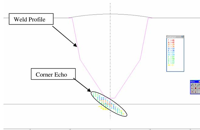
Figure 11 - Experimental results for inspection of Defect 1 with a single crystal transducer.
