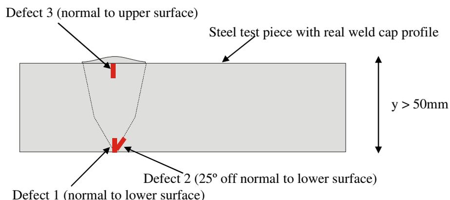
Figure 2 - Steel test piece showing defect locations and real weld cap surface profile
