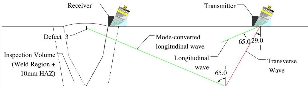
Figure 7 - Schematic of the Transverse-Longitudinal-Longitudinal mode conversion inspection of Defect 3 using pitch catch arrangement of single crystal transducers.
