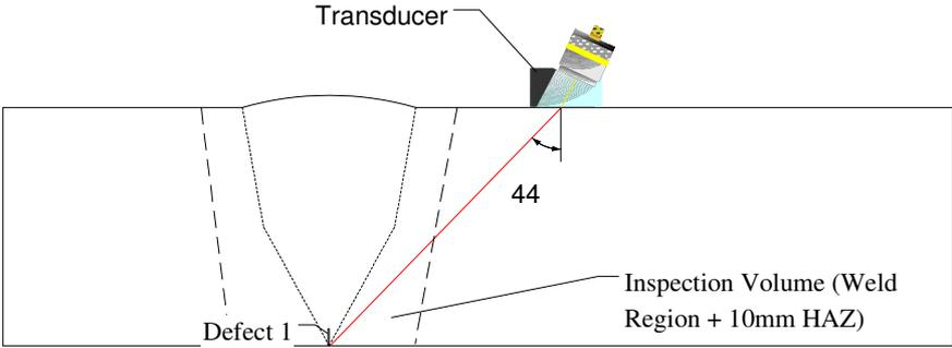
Figure 3 - Schematic of pulse echo shear wave inspection technique of Defect 1 (lack of root fusion) using a single crystal transducer.
