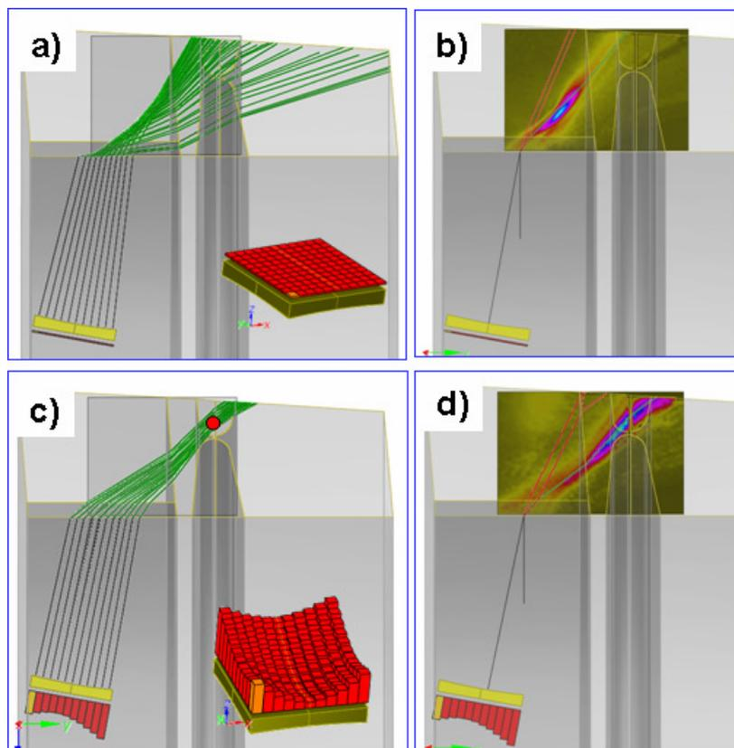
Figure 3 - Example of ray tracing and beam computation for a matrix phased array used to focus through a bimetallic weld.
