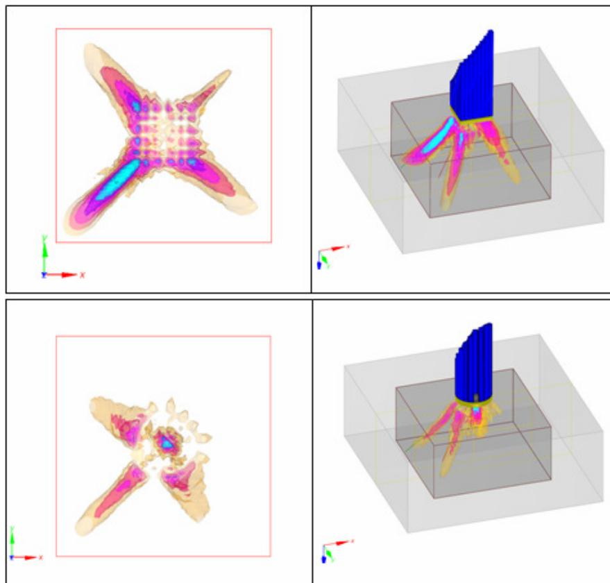
Figure 2 - Example of 3D beam computation with 2D splitting array patterns (2D matrix array of 8x8 elements, top view, and sectored arrays of 61 elements, bottom view).
