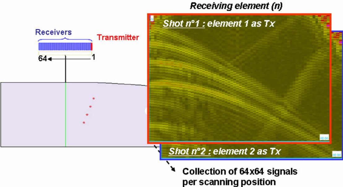
Figure 5 - Examples of signals acquired by the array, using the full matrix capture acquisition.
