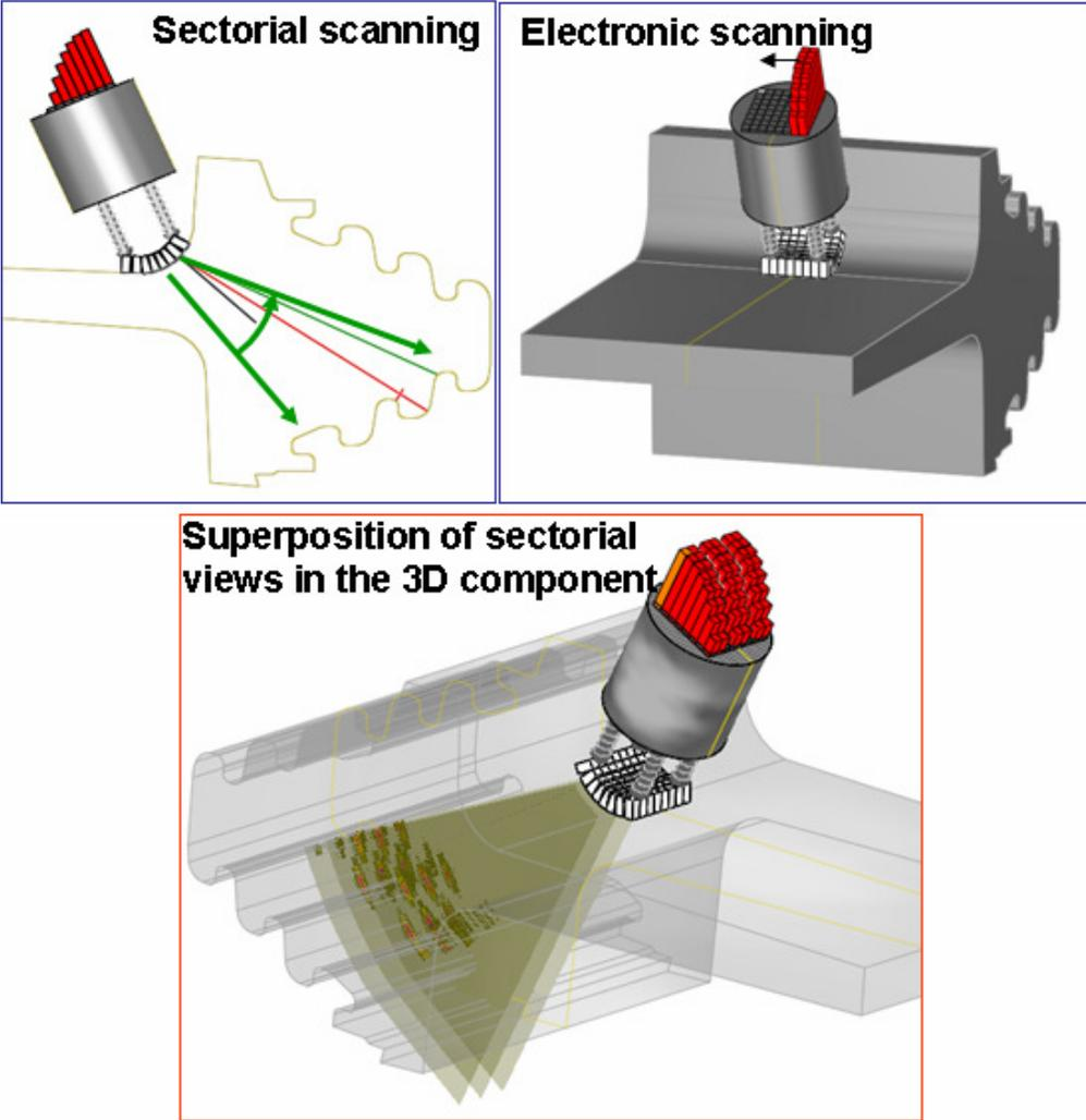
Figure 4 - Illustration of a phased array inspection technique combining electronic scanning and sectorial scanning over a turbine blade attachment and display of three simulated scans.
