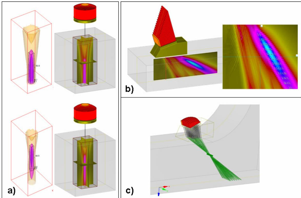
Figure 1 - Tools for evaluating phased arrays techniques: a) measure of the focal spot, b) estimation of the actual refraction angle, and c) ray tracing tool.
