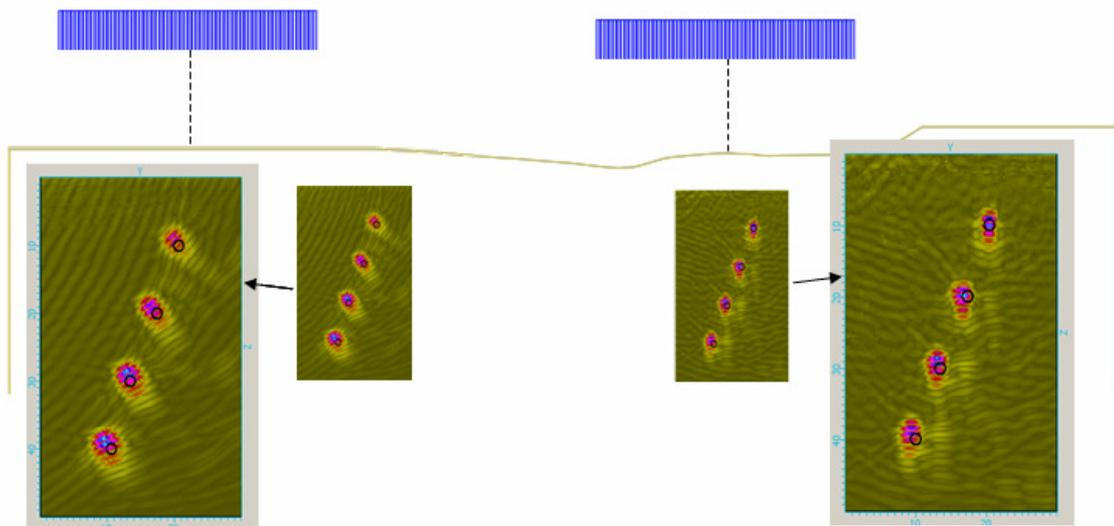
Figure 6 - Reconstruction over planar and irregular parts of the component.
