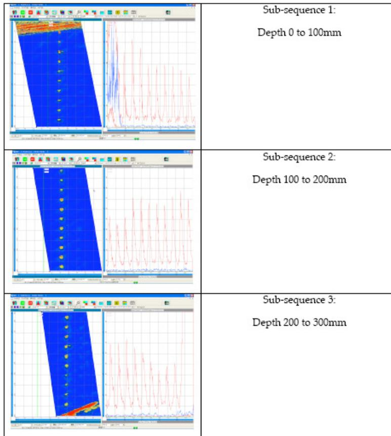
Figure 11 - Depth of field with 5MHz probe in Volume Focusing mode.
