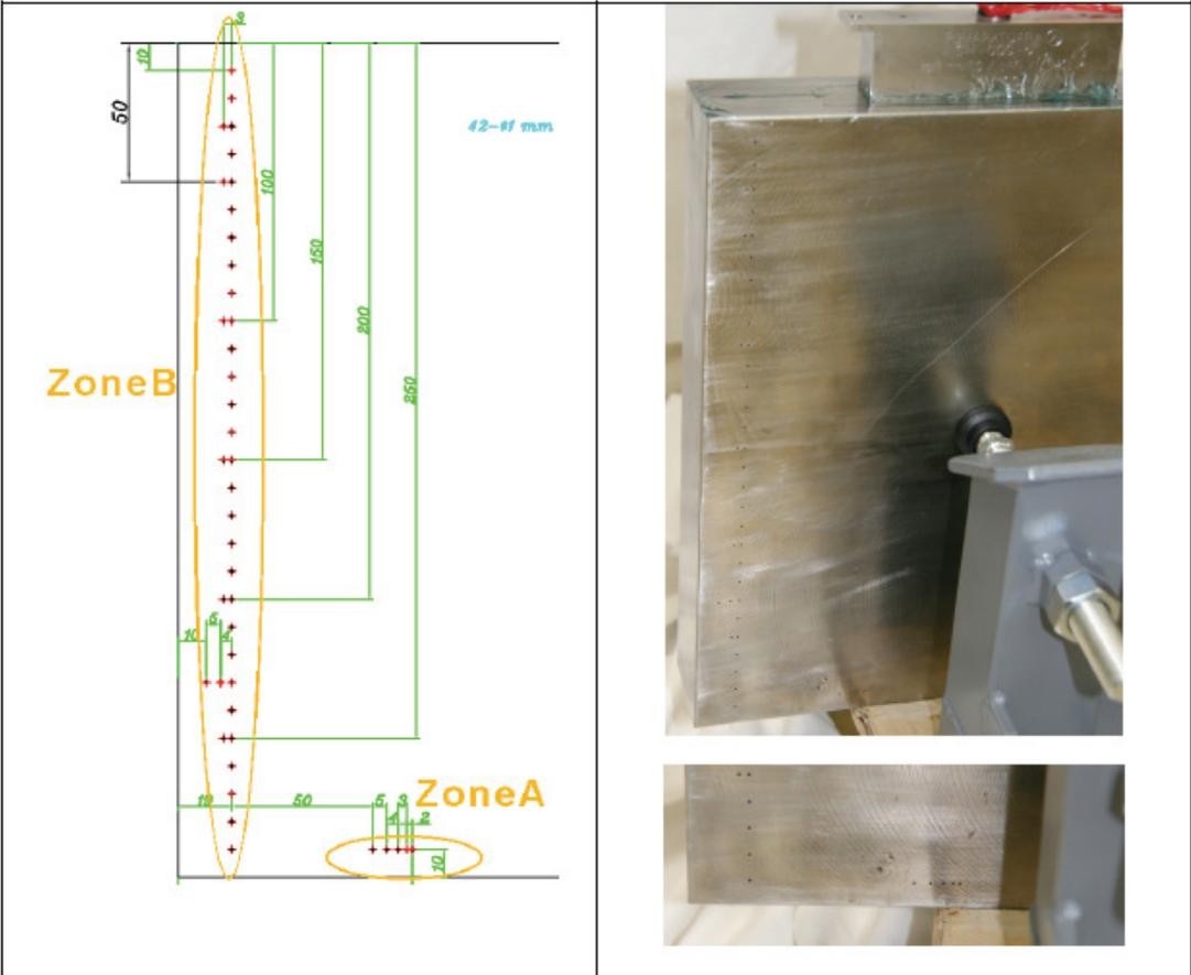
Figure 1 - Drawing and photo of the sample test piece used for experimentation
