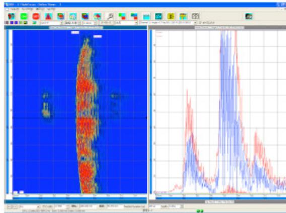
Figure 10 - Zone A in Volume Focusing mode, 5MHz probe
