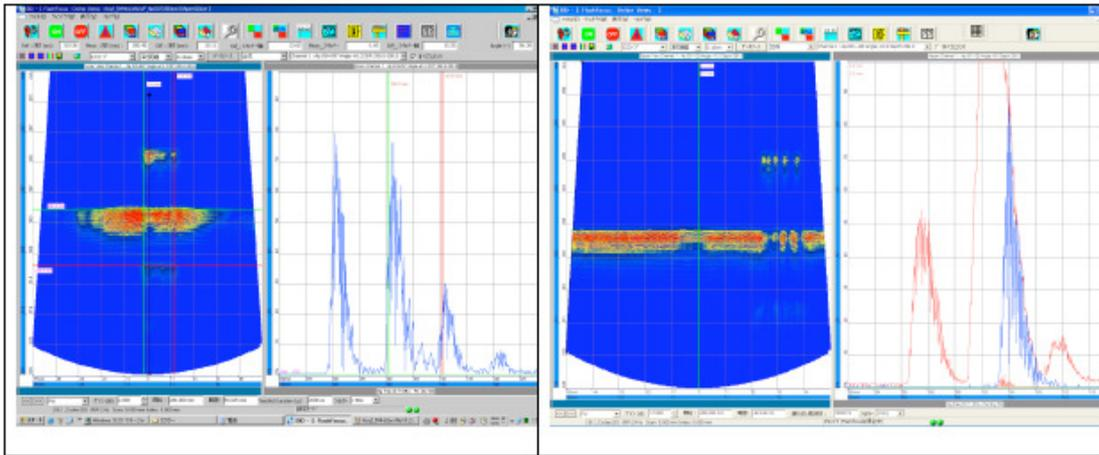
Figure 3 - Left: 64-element aperture. Right: 128-element aperture.
