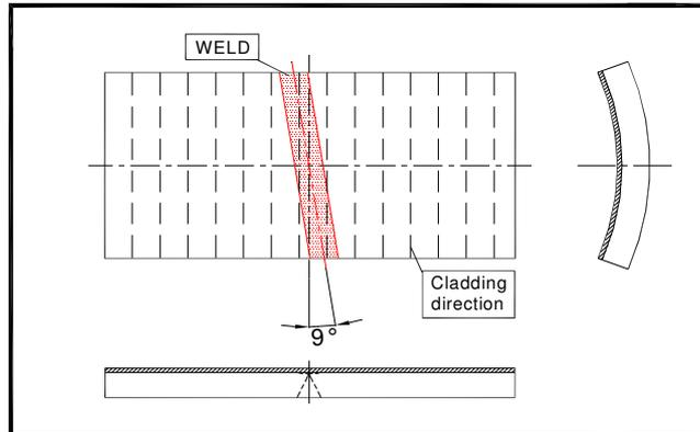
Figure 4 - Oblique weld in pipe connection and cladding beads direction.
