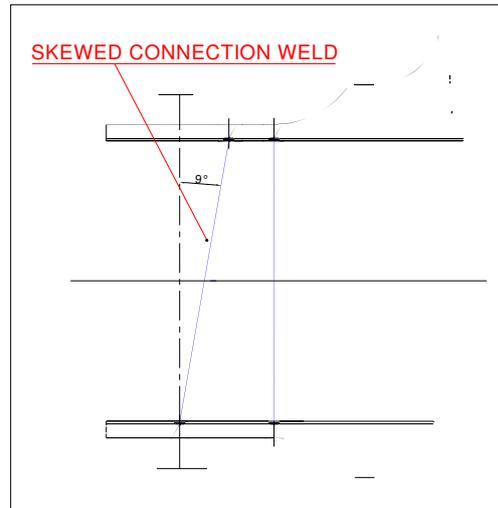
Figure 7 - Skewed weld in a nozzle to pipe connection
