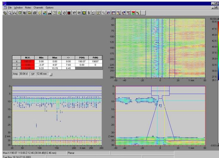
Figure 1 - Location of the weld centre line with a zero degree probe.
