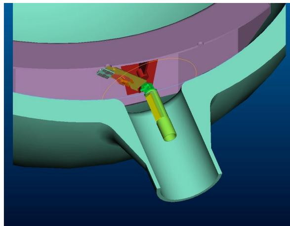
Figure 8 - Study of interferences in nozzles using modelling software.
