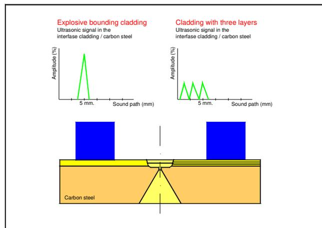
Figure 3 - Two different types of cladding at both sides of a pipe weld.
