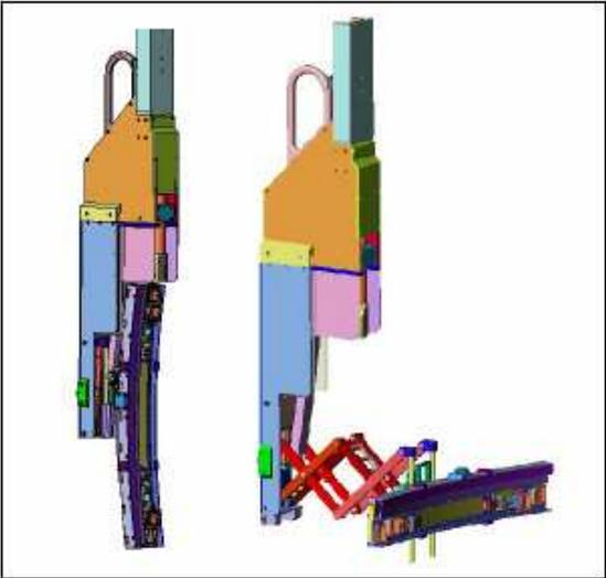
Figure 2 - CSIT folded for installation (left) and operating configuration (right)
