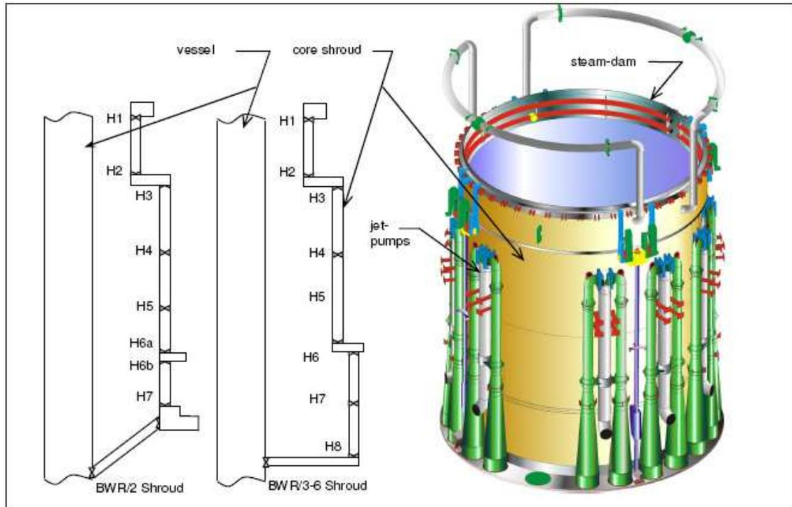
Figure 1 - Typical BWR shroud arrangement and weld configuration
