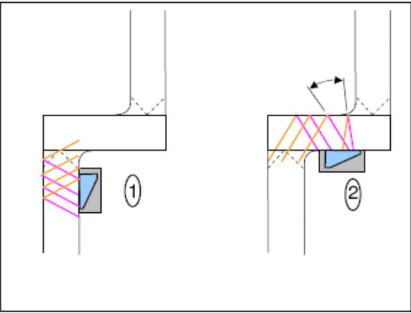
Figure 5 - PA inspection of H3 ring segment weld
