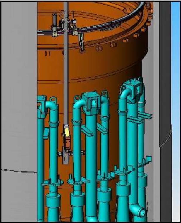
Figure 3 - Ring and cart with mast extending between jet-pumps
