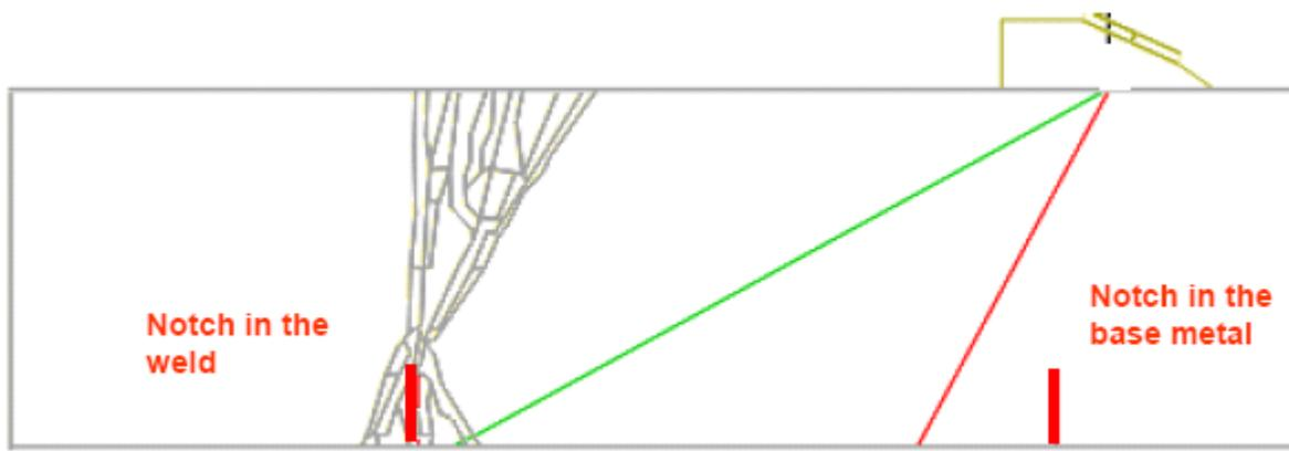
Figure 9 - Configuration of inspection of a notch located in the weld
