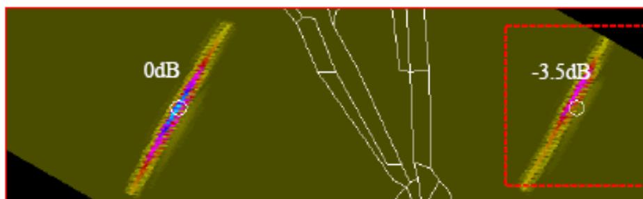
Figure 8 - Simulated Bscan image for the detection of a side drilled hole (without attenuation)
