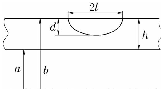
Figure 8 - Outer surface semi-elliptical crack
