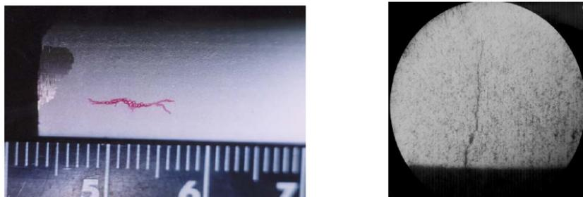
Figure 1 - Defect at steam generator PGV-1000 tube of VVER
