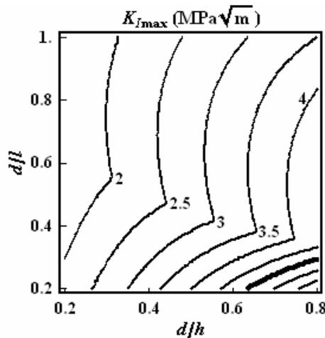
Figure 11 -  $K_{I\max}$  dependence on the crack dimensions (location at the middle of the tube)
