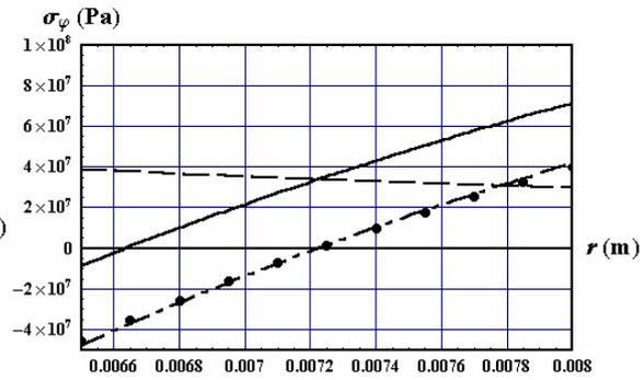
Figure 7 - Circumferential stresses distribution with wall depth at the middle part of the tube (5m from tip)
