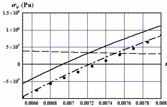
Figure 6 - Circumferential stresses distribution with wall depth at tube tip
