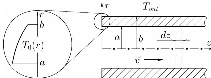
Figure 2 - Temperature field problem for heat-exchange tube
