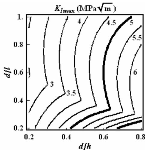
Figure 10 -  $K_{I\max}$  dependence on the crack dimensions (location closed to tube tip)
