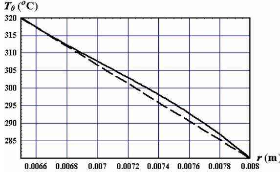
Figure 4 - The initial temperature profile in the wall of the tube
