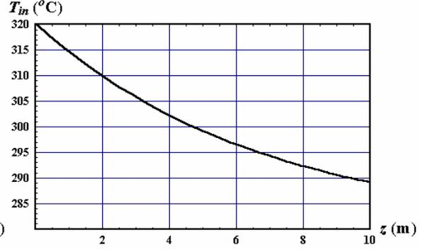
Figure 5 - Inner surface temperature distribution along tube length
