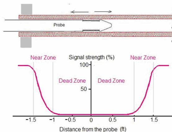
Figure 5 - General pattern of GW signal strength in DZ and NZ areas for 200 kHz probe
