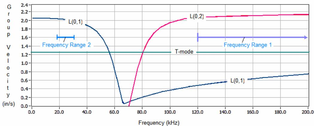
Figure 3 - Group velocity of different modes of GW in 1" OD SeaCure tubing
