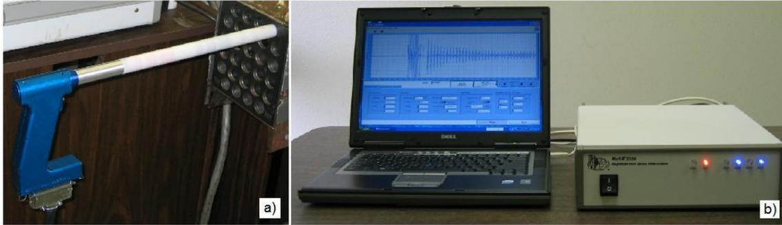
Figure 2 - GW probe (a) and MsS Instrument (b)
