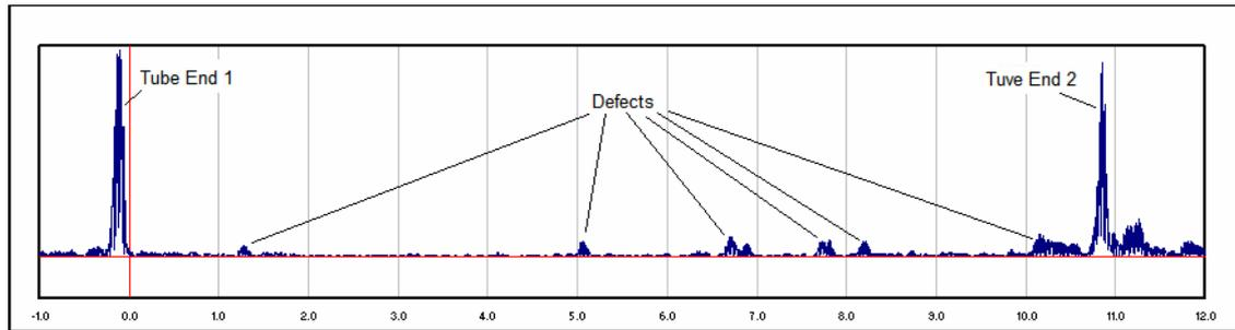
Figure 8 - 'A'-scan presentation with 100% coverage of the tube length
