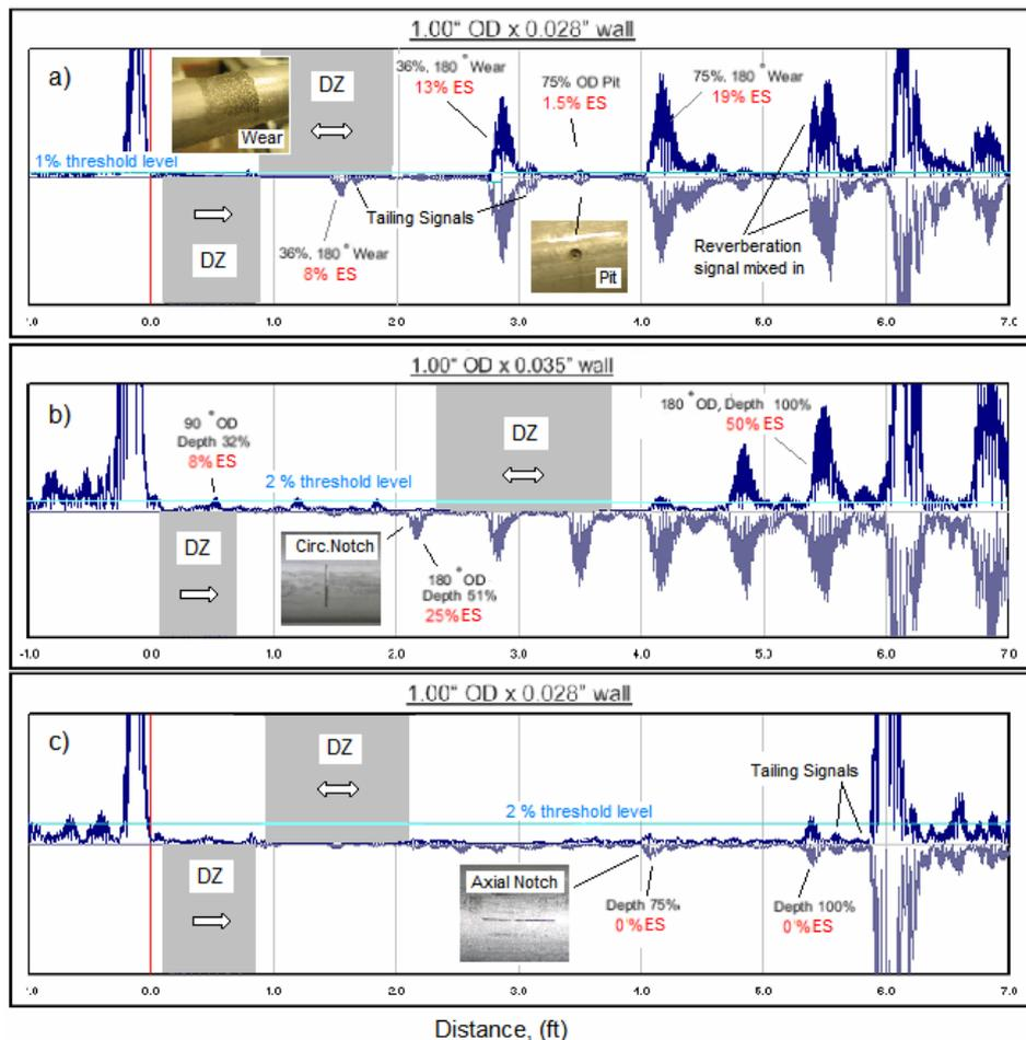
Figure 10 - Data obtained from tubes with different flaws using L(0,2) mode of GW at 250 kHz:
