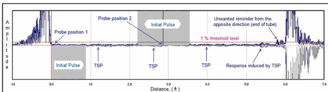
Figure 9 - Typical pattern of the responses obtained from SeaCure tubing containing no defects
