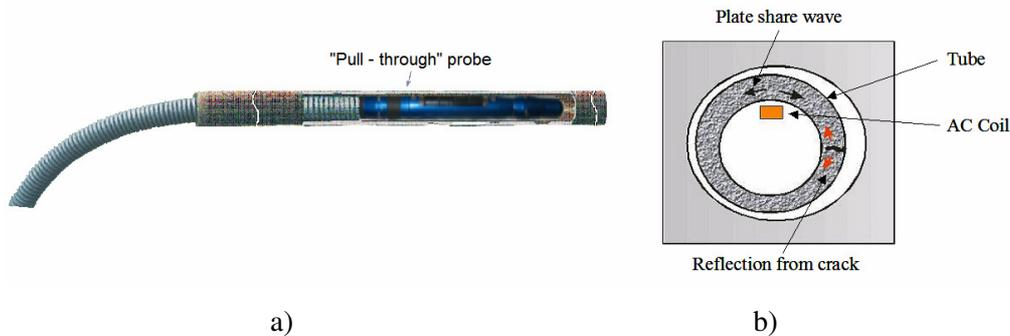
Figure 11 - Plate SW probe: (a) "pull-through" type of instrument used for detection of AXC;
