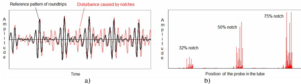
Figure 12 - Detection of small volume AXC: (a) a disturbance induced to the reference signal by axial notch; (b) processed signal providing an indication of the severity of the disturbance produced by 32, 50, and 75% deep and 0.005" wide axial notches
