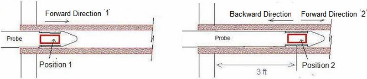
Figure 6 - Principle of data acquisition using GW probe: fast screening mode (left); full screening mode (left plus right)
