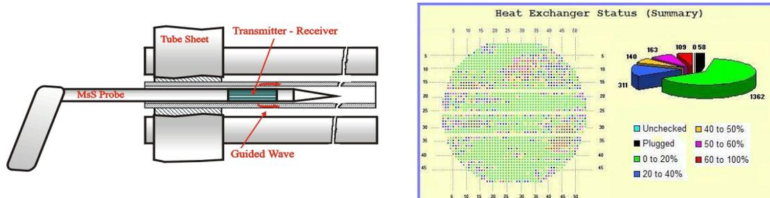
Figure 1 - Concept of screening using GW:
