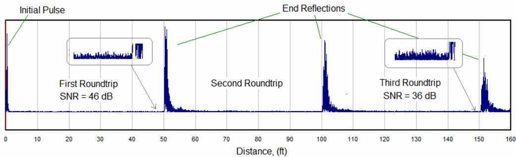
Figure 4 - Data obtained from clean 50 ft long 1" OD SeaCure tube
